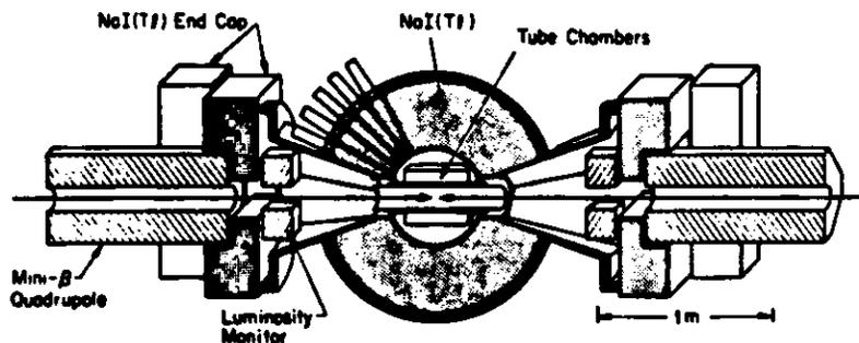
Figure 4. The main components of the Crystal Ball at DORIS II
