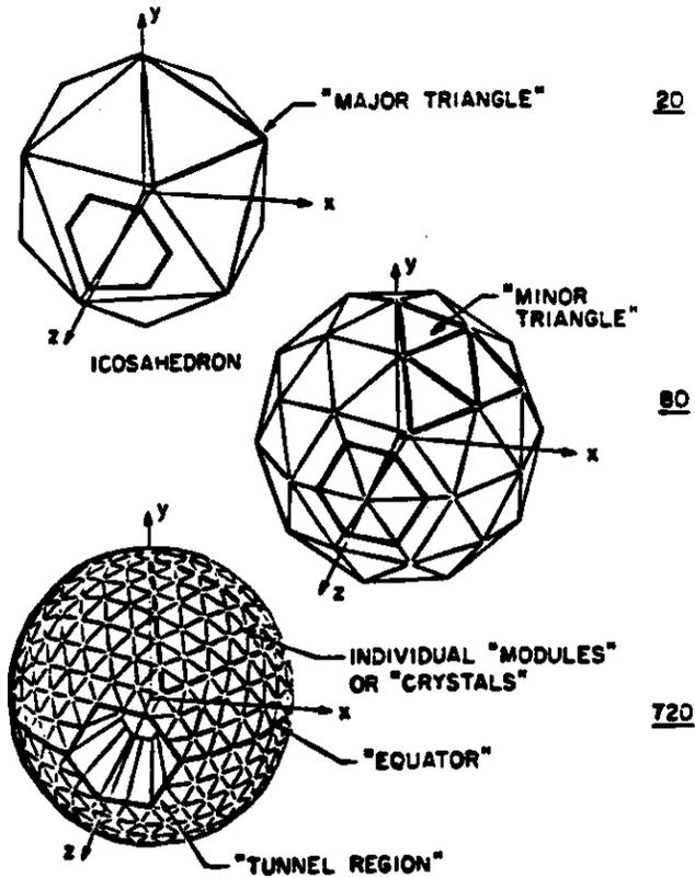
Figure 5. CB geometry and nomenclature (from /OREG80/)
