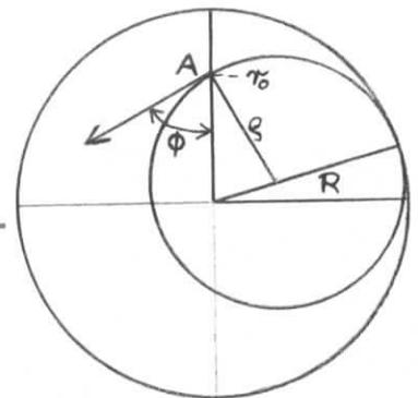
In the fringe field the positrons get an azimuthal momentum  $\Delta p = p_0 \sin \Delta \phi$  while the radial momentum  $p_r = p_0 \sin \phi_r$  remains constant.
