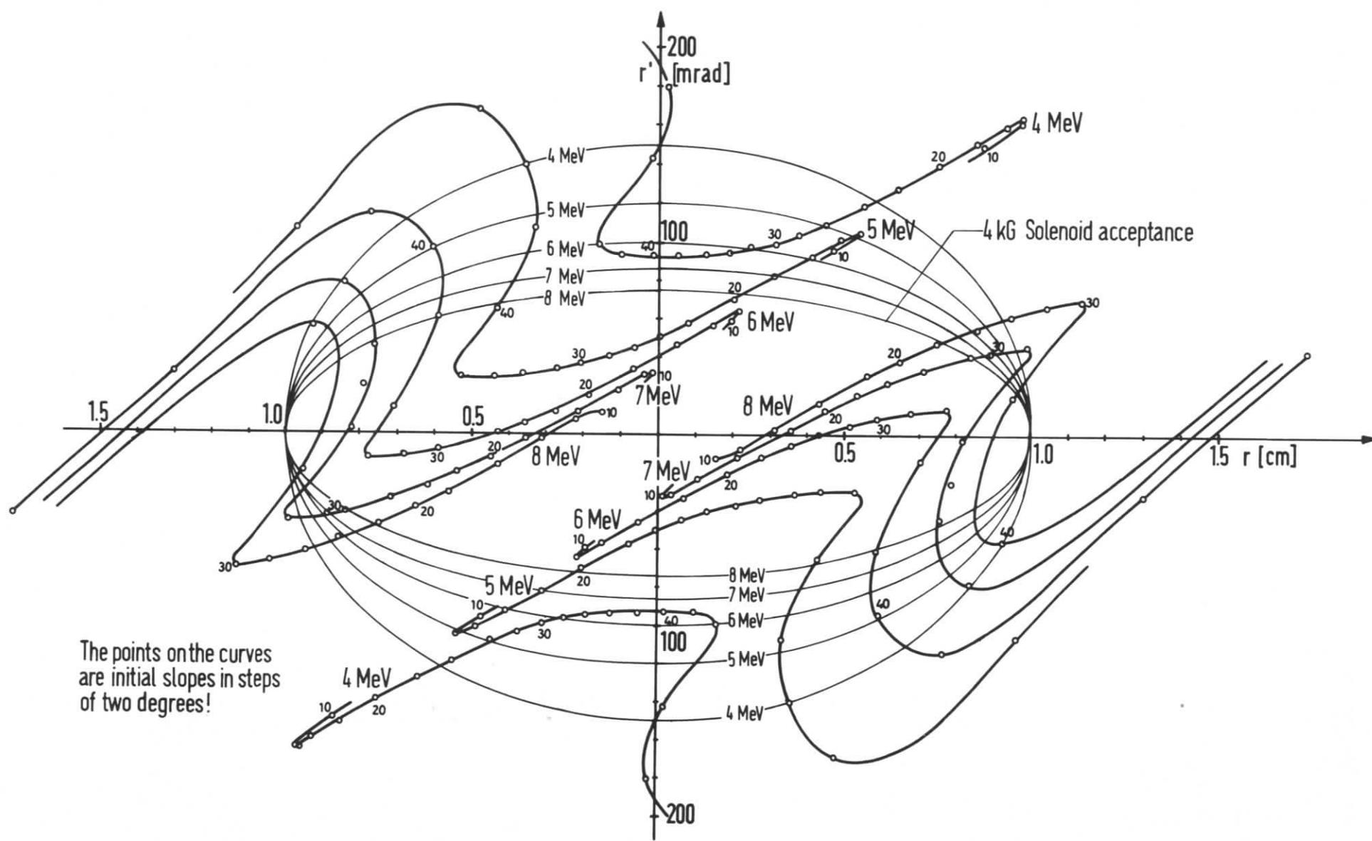
fig.7 Emittance of the Positron Horn for Various Positronenergies at Z=8 cm
