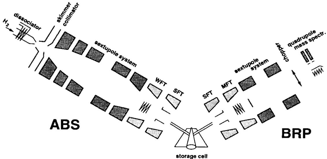
Figure 3.4: Schematic picture of the polarized hydrogen target.
