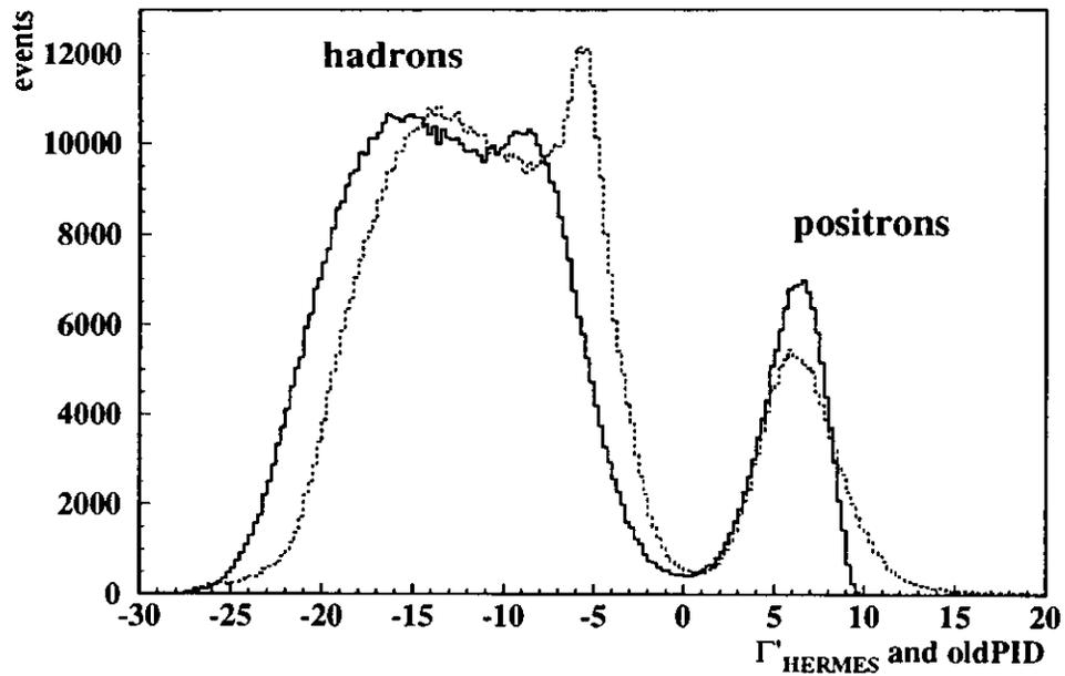
Figure 4.12: PID5  $\Gamma'_{\text{HERMES}}$  (solid line) and the old PID scheme (dashed line) for good PID runs from 4611-5120 (multiplicity > 1, caused by the limited database used.)
