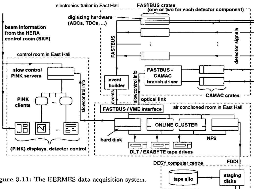
Figure 3.11: The HERMES data acquisition system.
