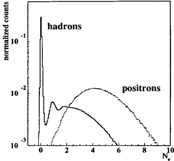
Figure 3.7: The normalized Čerenkov response for hadrons (solid line) and positrons (dashed line) from 1996 data integrated over all momenta.
