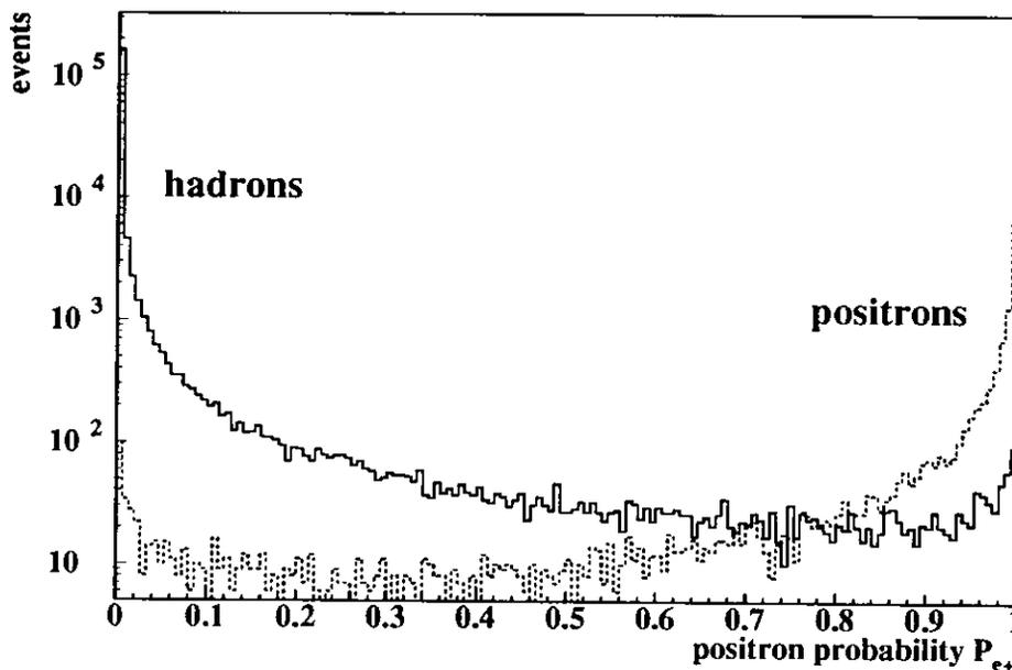
**Figure 4.10:** Result of the probability analysis: the positron probability  $P_{e+}$  given by the TRD likelihood method for runs 4216-4240. For the distinction of hadrons (solid line) and positrons (dashed line) see tab.4.2.
