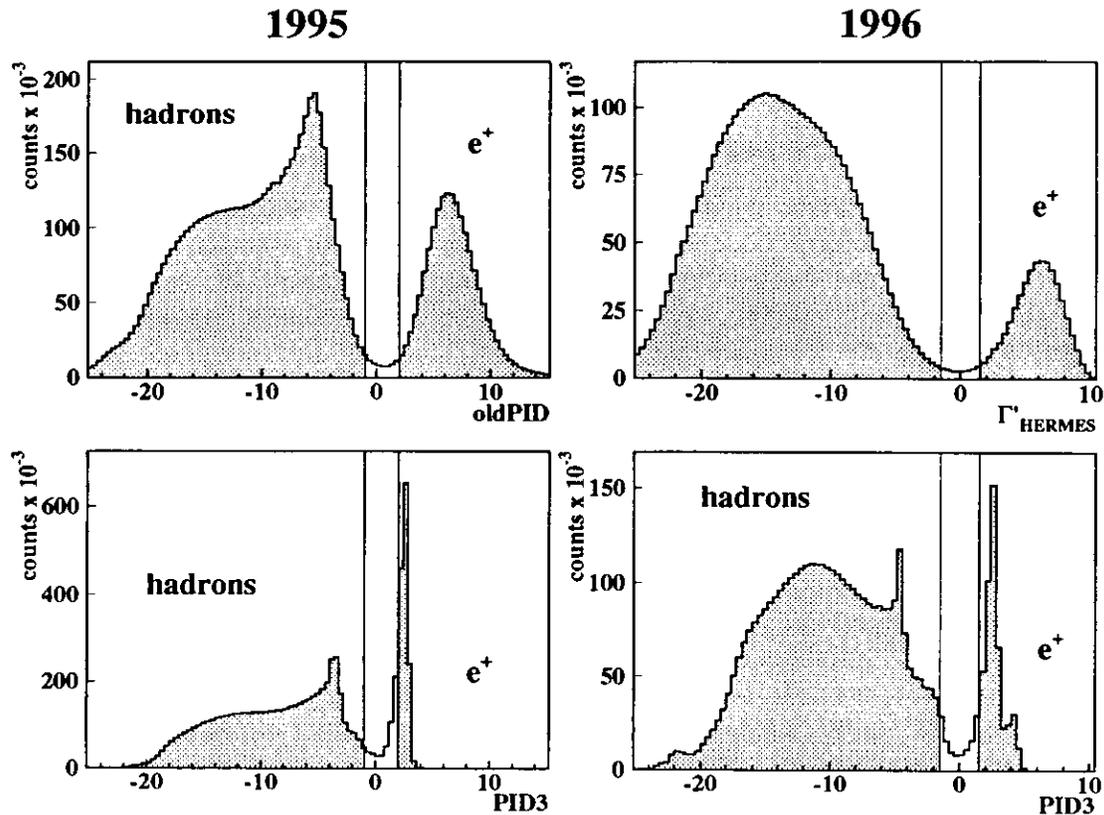
Figure 5.5: The PID schemes used for hadron and positron identification for 1995 and 1996. Top: All detectors. Bottom: PID downshifting used (PID3) in case of a bad the TRD. The cuts applied are indicated by vertical lines.
