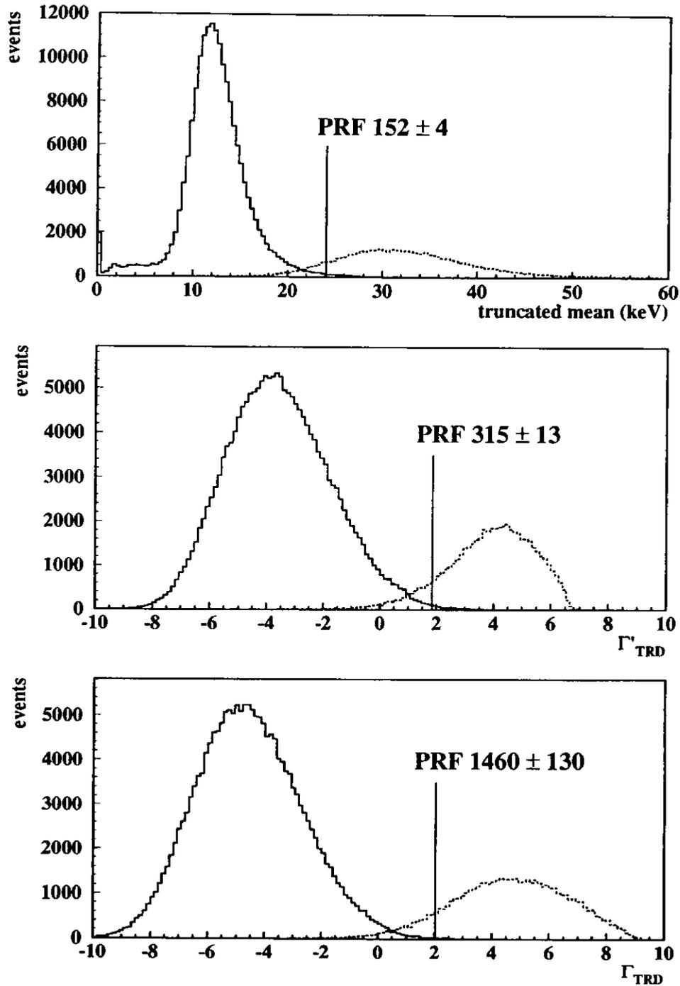
**Figure 4.11:** Truncated mean and logarithmic likelihoods ( $\Gamma'_{TRD}$  and  $\Gamma_{TRD}$ ) for runs 4216-4240. For the separation of hadrons (solid line) and positrons (dashed line) see tab.4.2. The cut for 90% positron efficiency for the calculation of the PRF is indicated by a vertical line.
