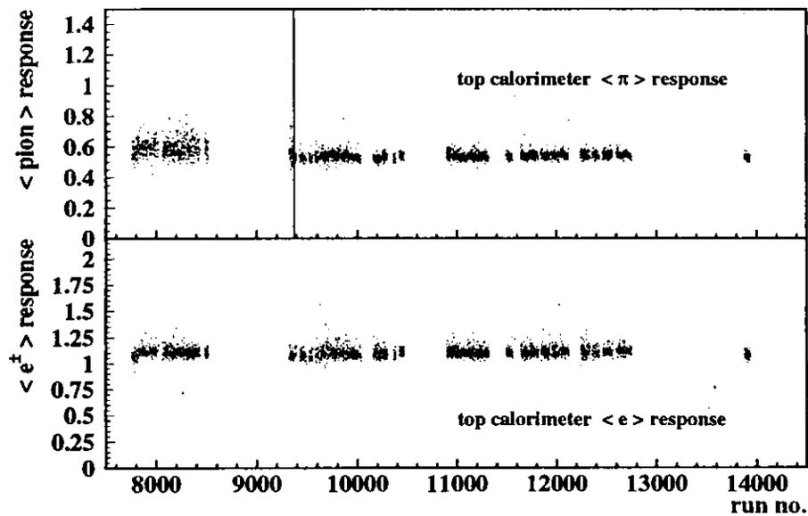
Figure 7.4: The average calorimeter response for hadrons and  $e^\pm$  versus run number (1996). The horizontal line marks the point in time the calorimeter threshold was changed from 3.5 to 1.4 GeV.
