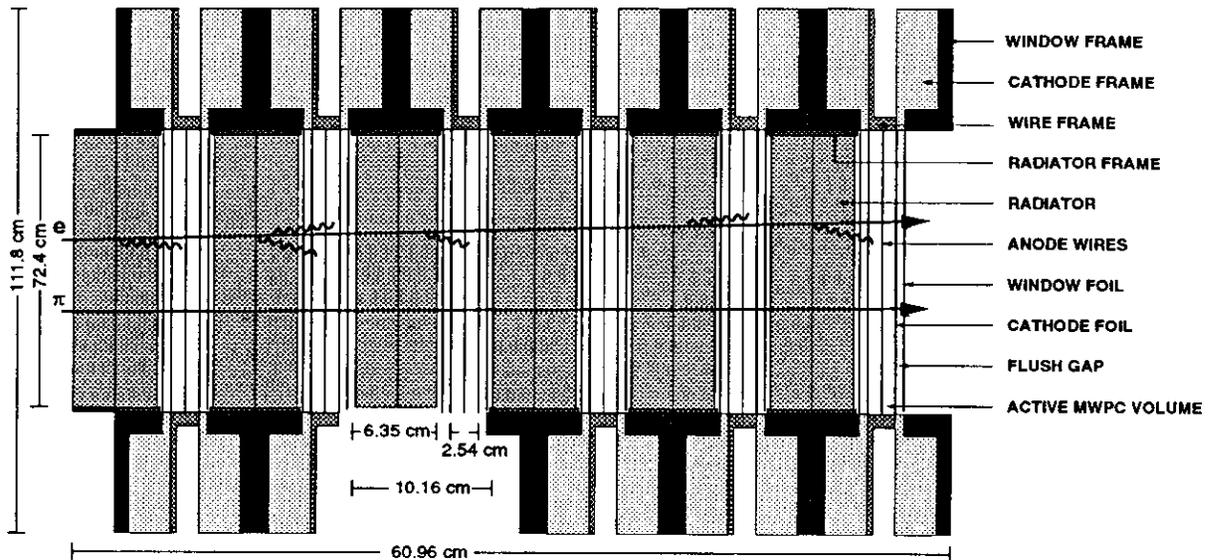
**Figure 4.2:** One half of the HERMES Transition Radiation Detector. The opening angles of the transition radiation photons emitted by the electron/positron are exaggerated.
