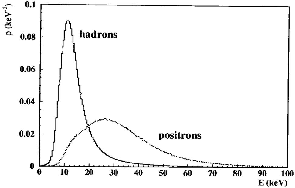
**Figure 4.8:** Parent distributions for module 1: normalized hadron response  $\rho_1^h$  for  $p \in [6; 8 \text{ GeV}]$  (solid line); normalized positron response  $\rho_1^{e^+}$  for  $p \in [6; 12 \text{ GeV}]$  (dashed line).
