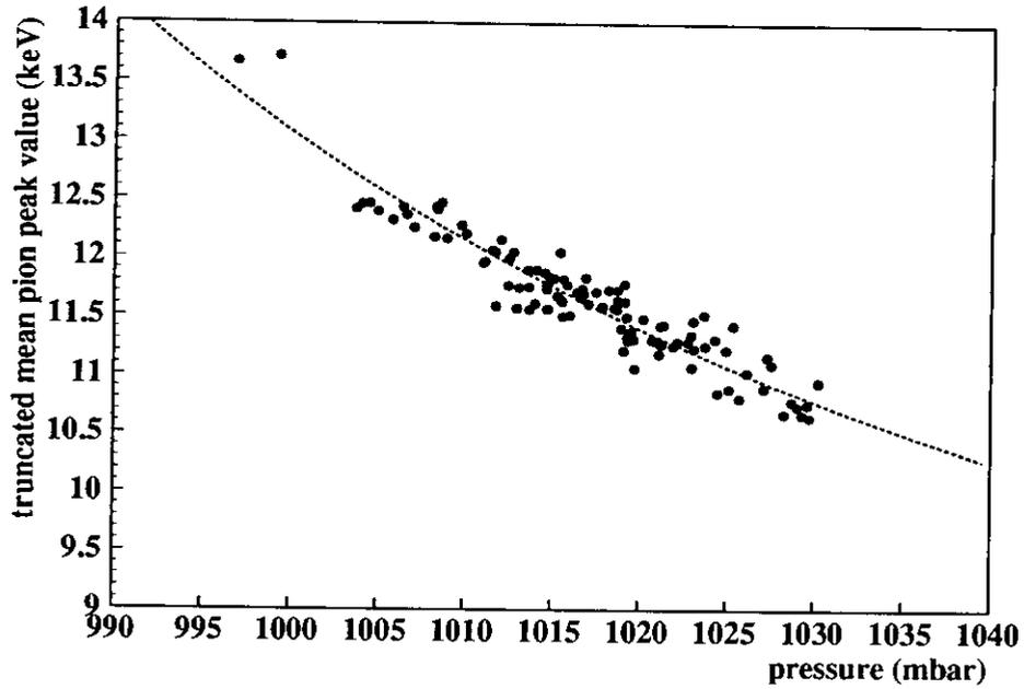
Figure 4.6: Non-calibrated pion peak position for 108 good runs versus atmospheric pressure with a hyperbolic fit  $f(p_{atm}) = \frac{771.5 \text{ mbar keV}}{p_{atm} - 913.32 \text{ mbar}} + 4.17 \text{ keV}$ .
