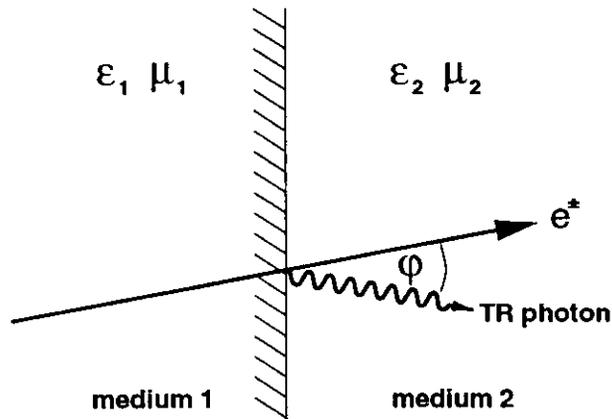
**Figure 4.1:** When a point charge passes the boundary between two dielectric media, it emits transition radiation (TR).
