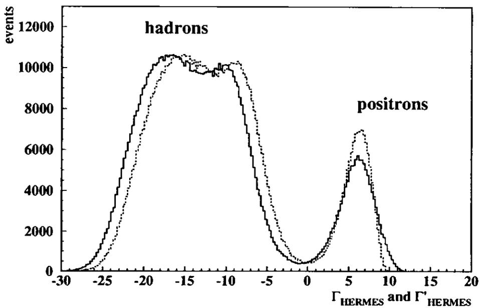
Figure 4.13: The overall PID value  $\Gamma_{\text{HERMES}}$  (solid line) in comparison with  $\Gamma'_{\text{HERMES}}$  (dashed line) for good PID runs from 4611-5120 (1995 data) (multiplicity > 1).
