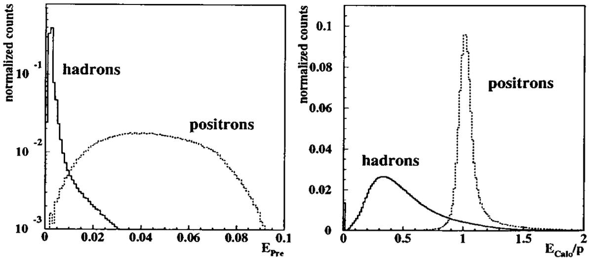
Figure 3.9: The normalized preshower (left) and calorimeter (right) responses for hadrons (solid line) and positrons (dashed line). The whole momentum range is shown (1996).
