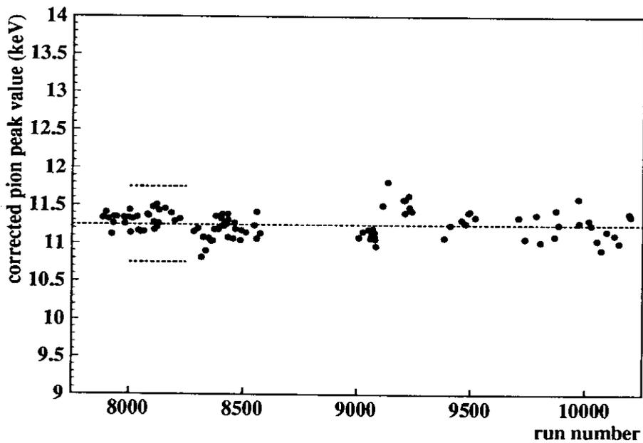
Figure 4.7: Corrected (non-calibrated) pion peak position for 108 good runs versus run number. Correction:  $peak_{corr} = peak - f(p_{atm}) + 11.25 \text{ keV}$ .
