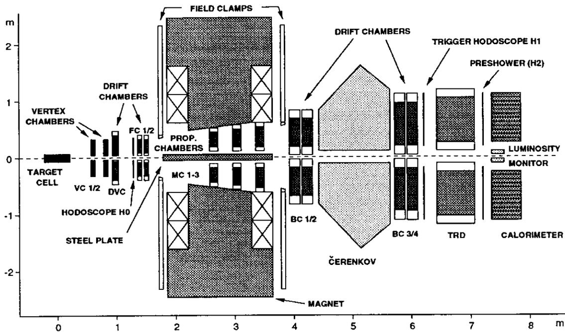
Figure 3.5: A schematic drawing of the HERMES spectrometer.
