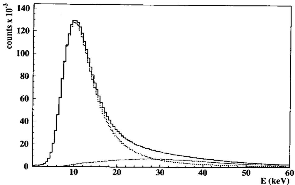
**Figure 4.3:** Response of TRD module number 3 from selected fills from 1996 (solid line). The response is the sum of a hadron (dashed line) and a positron (dotted line) contribution. The positron/hadron samples are determined by hard cuts on the other detectors (see tab.4.2).
