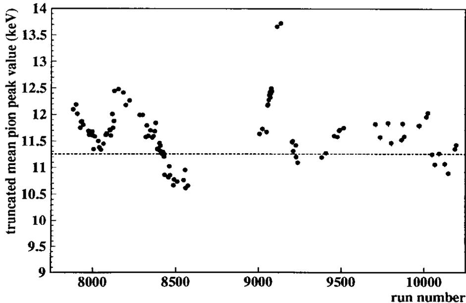
Figure 4.5: Non-calibrated pion peak position for 108 good runs versus run number (1996).
