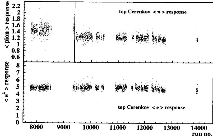
Figure 7.1: The average Čerenkov response for hadrons and  $e^\pm$  versus run number (1996). The horizontal line marks the point in time the calorimeter threshold was changed from 3.5 to 1.4 GeV.
