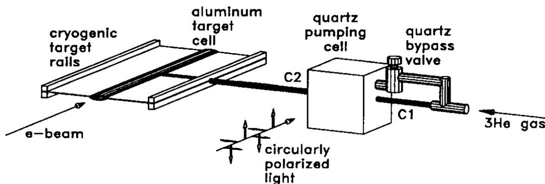
Figure 3.3: The optical  $^3\text{He}$  pumping system.
