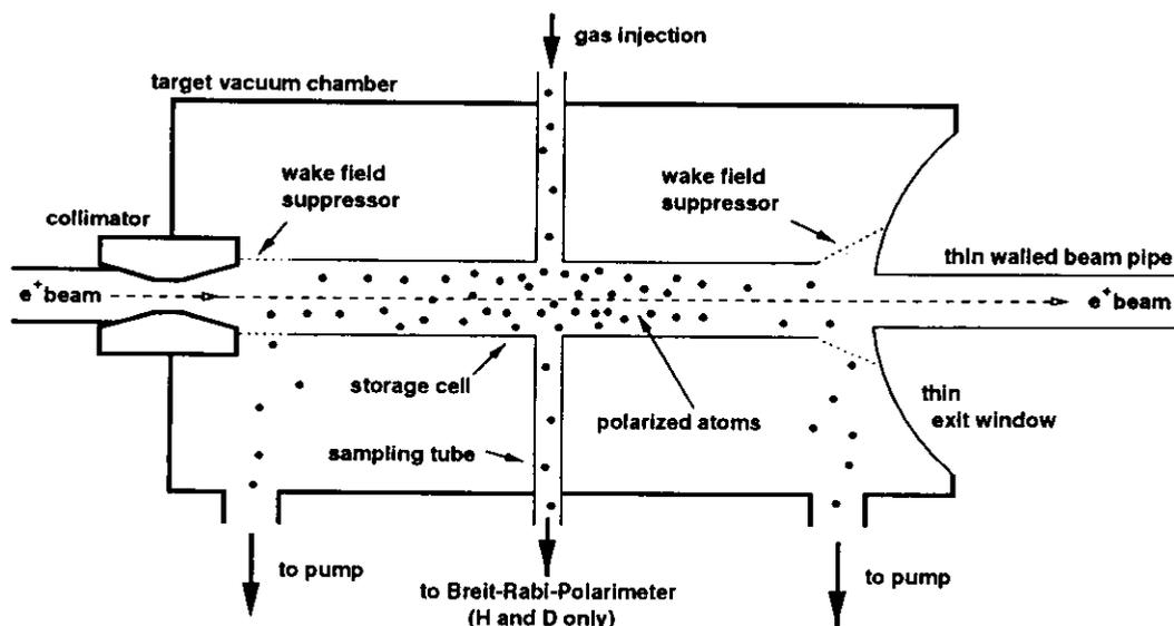
Figure 3.2: The internal gas target in the positron beam.
