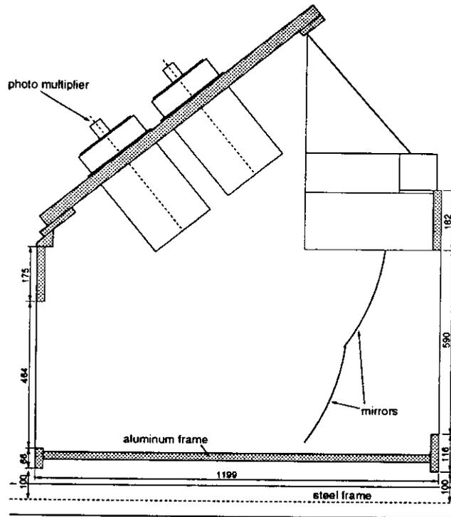
Figure 3.6: The upper threshold Čerenkov counter.
