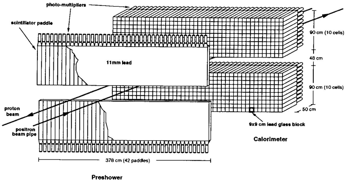
Figure 3.8: Perspective view of preshower detector and calorimeter.
