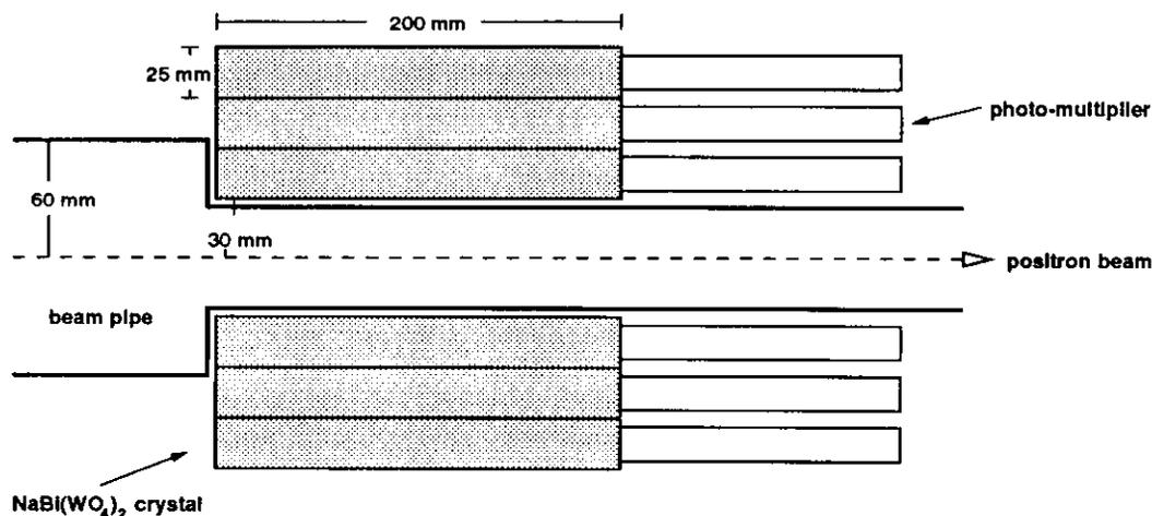
Figure 3.10: The HERMES luminosity monitor at the positron beam line.
