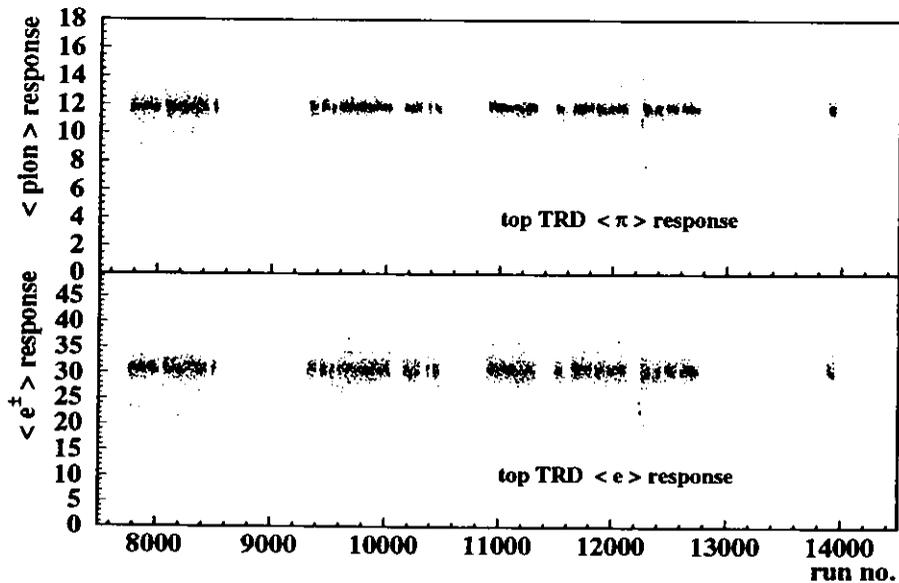
Figure 7.2: The average TRD response for hadrons and  $e^\pm$  versus run number (1996). The runs around 8000 and 12300 show a high-voltage trip. In these runs, the TRD is not used for particle identification (PID-downshifting).
