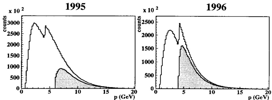
Figure 5.6: Kinematic distribution of all measured hadrons (empty histogram) with the fraction of all identified pions (grey area). The benefit of the lower Čerenkov threshold in 1996 is clearly visible as an increase in the pion identification efficiency. The marked decrease around 3.5 GeV is an effect of the calorimeter threshold.
