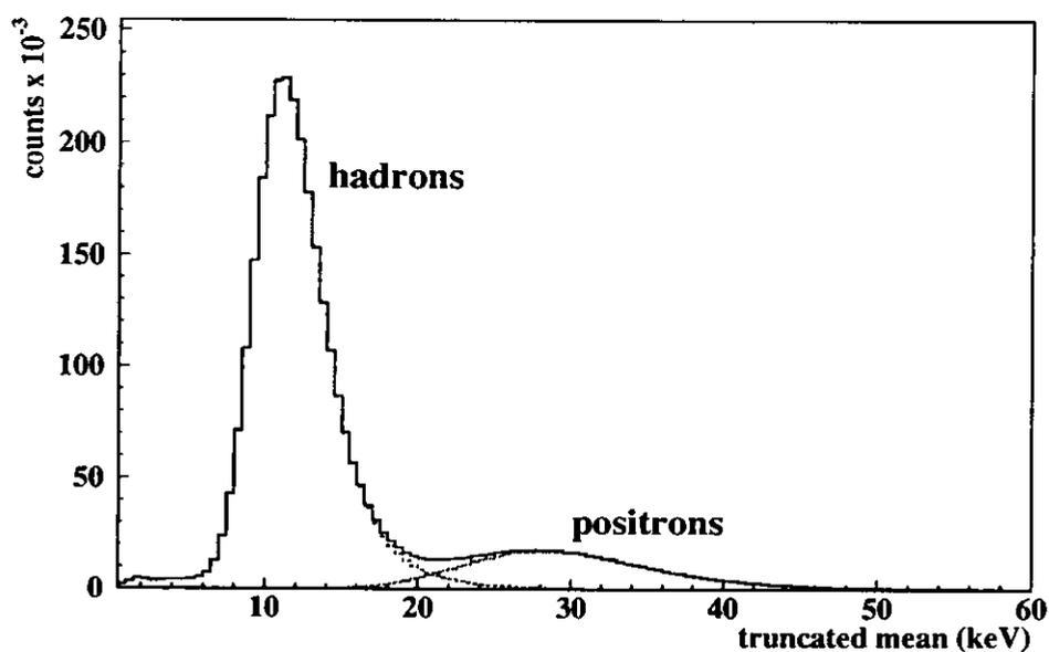
**Figure 4.4:** Truncated mean of the six TRD modules from selected fills from 1996 (solid line). The hadron response is displayed as dashed line, the positron response as dotted line. Both samples are determined by hard cuts on the other detectors (see tab.4.2).
