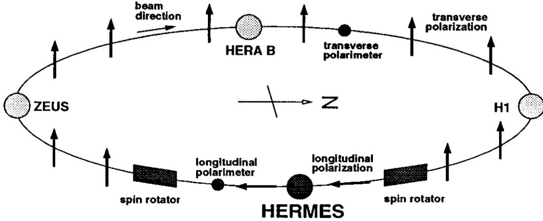
**Figure 3.1:** The HERA positron ring with spin rotators in Hamburg, Germany. The arrows indicate the direction of the beam polarization.
