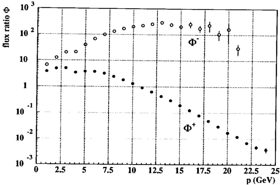
**Figure 4.14:** The flux ratios  $\Phi^+$  (solid circles) and  $\Phi^-$  (empty circles) obtained by an Bayesian iteration using  $\Gamma'_{\text{HERMES}}$  and all good PID runs from 1995 (multiplicity > 1 and  $\Theta \in [40; 70 \text{ mrad}]$ ).
