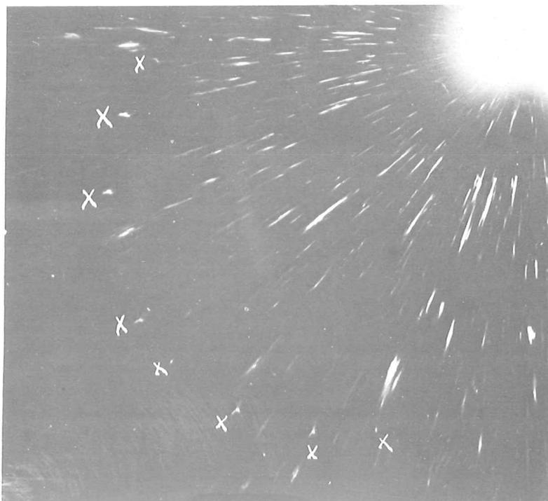
Fig. 3 Laue photograph of the sample of Fig. 2 at a higher temperature, after recrystallization. Some reflexions belonging to the same Laue zone are marked by x.
