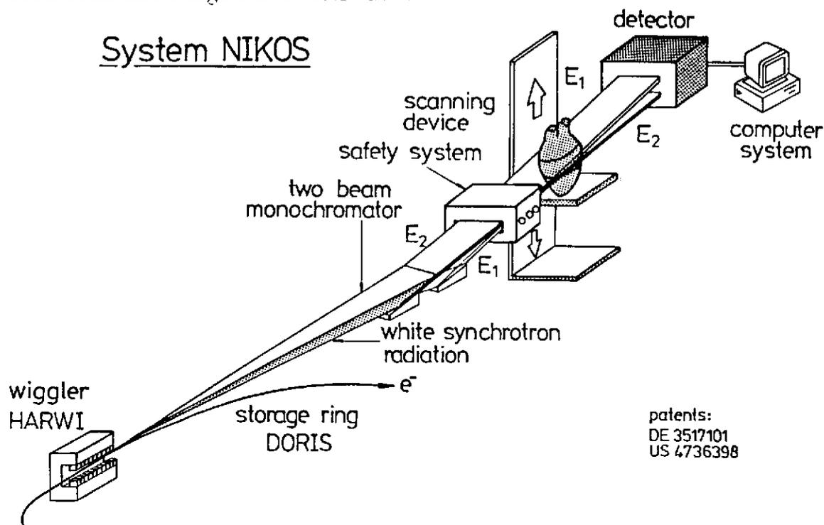
Figure 2: Schematic diagram of the system NIKOS II.
