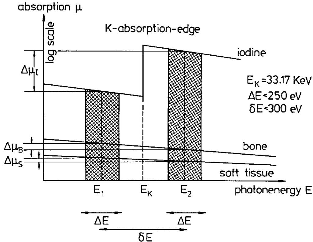
Figure 1: K-edge of iodine at  $E_K = 33.17 \text{ keV}$ .  $E_1$  and  $E_2$  denote the two energies of the quasi-monochromatic beams for dichromography with bandwidth  $\Delta E$ .
