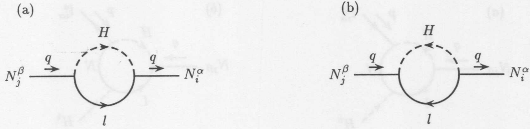
Figure 1.1: Leading order contributions to the self-energy of the heavy Majorana neutrinos. The fermion flow has been chosen parallel to the external momentum q .
