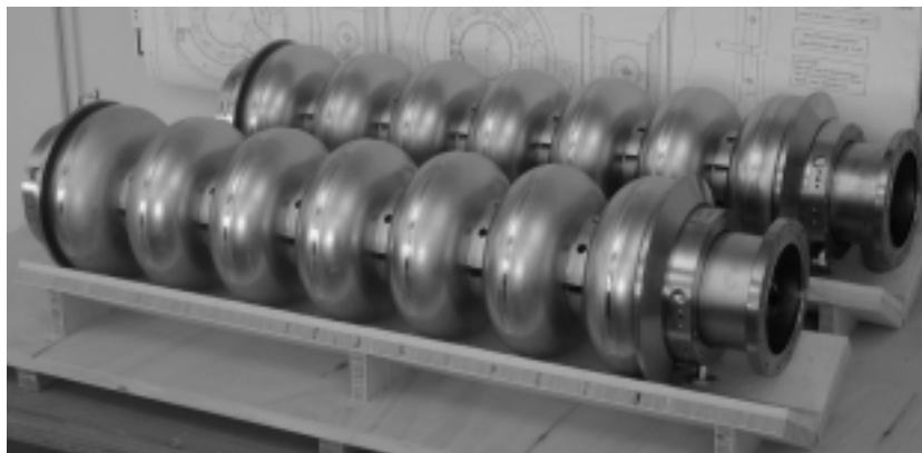
Figure 10.1: Niobium 7-cell cavities for the 2 \times 7 -cell prototype superstructure.
