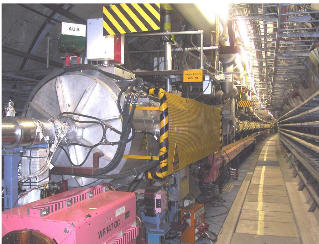
Figure A.28: The two 52 MHz cavities build up the proton buckets at the injection energy of 40 GeV.
