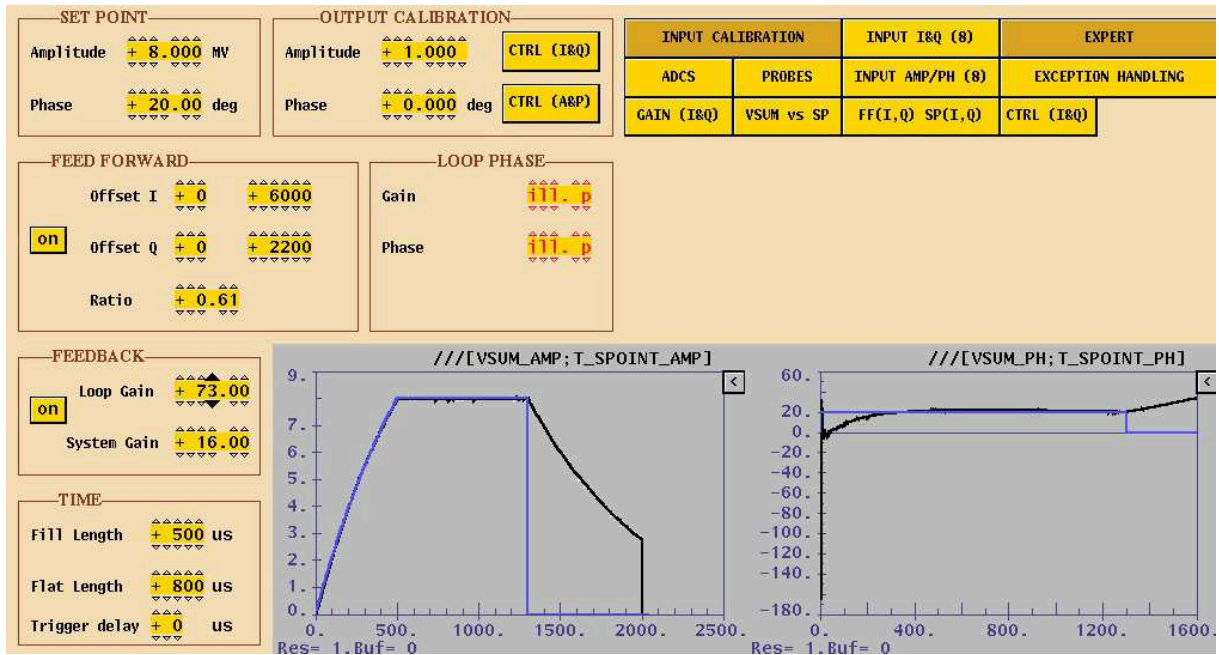
Figure 30: Main panel of the server. The SIMCON is running with Feedforward and feedback.
