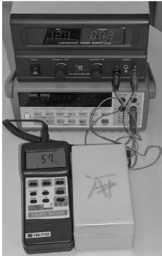
Figure 12: Prototype test system for COTS LED fast neutron dosimeter
