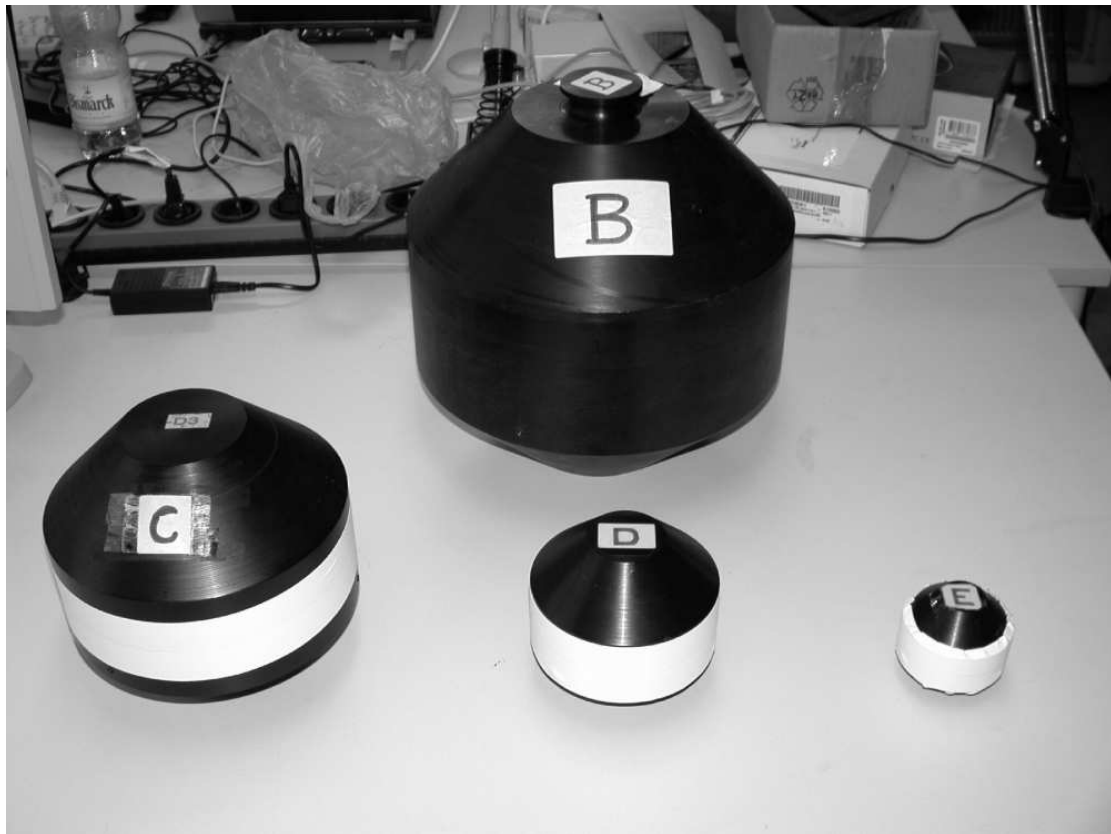
Figure 25: Polyethylene spheres for LEDs radiation experiments in Linac II tunnel
