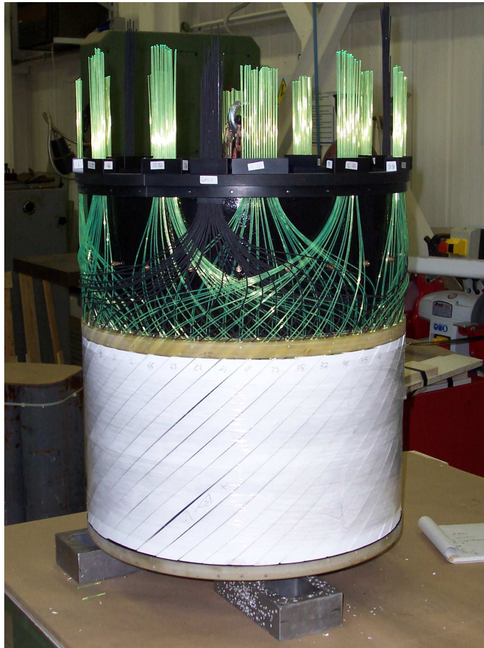
Figure 4.11: The photon detector during its assembly. The scintillator strips of the outer layer are visible, as are the wavelength shifting fibres and the connector ring.
