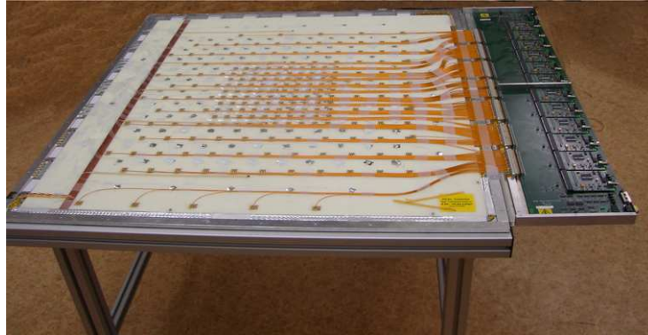
Figure 2.11: Picture of an opened AHCAL module with readout electronics.
