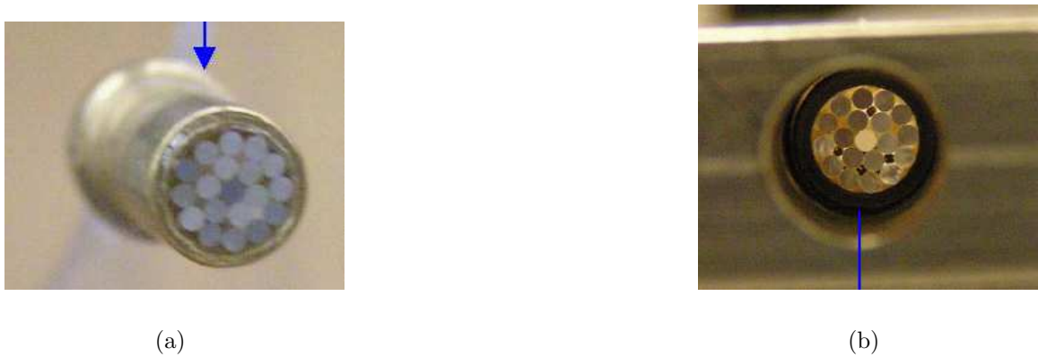
Figure 5.6: (a) A glued light guidance fibre bundle surrounded by a metal sleeve. (b) The same bundle fixed centric in a module by the metal sleeve.
