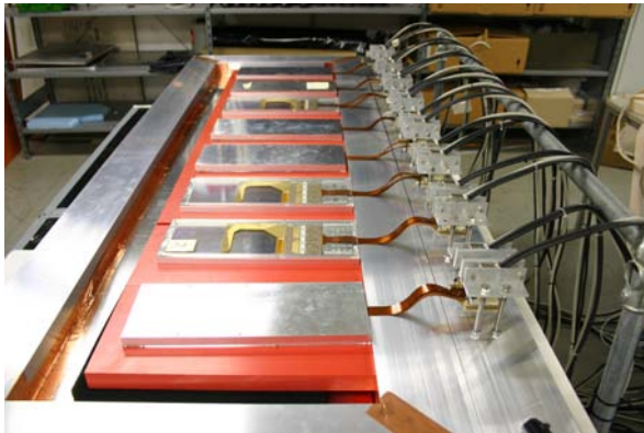
Figure 8.1: Photo of the bench test setup. Eight modules are placed on plastic plates to prevent capacitive coupling to the aluminium plate beneath. During the tests a light tight box was placed on top of the setup.
