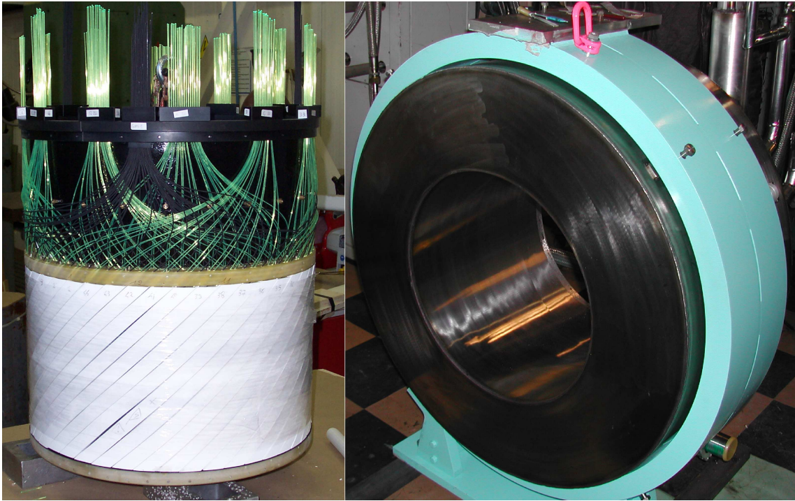
Figure 4.6: Photographs of the Photon Detector (left) and the magnet (right). The photon detector fits flush inside the bore of the magnet in the final assembly.
