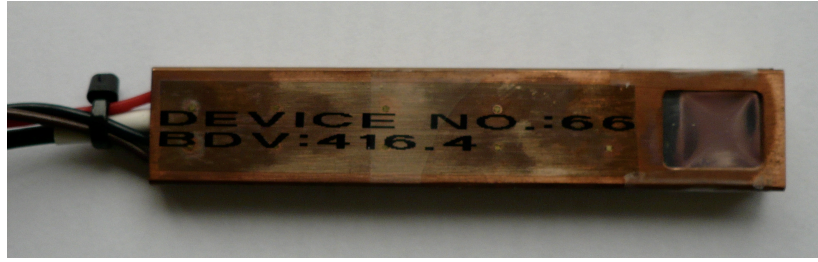
Figure 3.14: Amplifier and APD head with an active area of 10 \times 10 \text{ mm}^2 .
