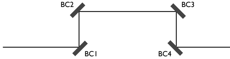
Figure 4.1: Crystal arrangement of the delay unit in the symmetric four crystal Bragg configuration.
