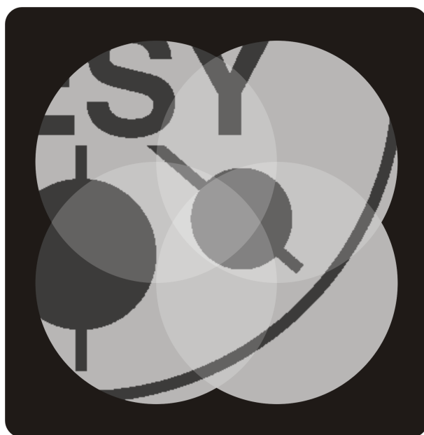
Figure 2.22: Schematic drawing of the ptychography-method. A sample is illuminated with a homogeneous circular intensity distribution. If the diffraction pattern is known for every individual illumination function the phase problem can be solved by the described ptychographic phase retrieval method.
