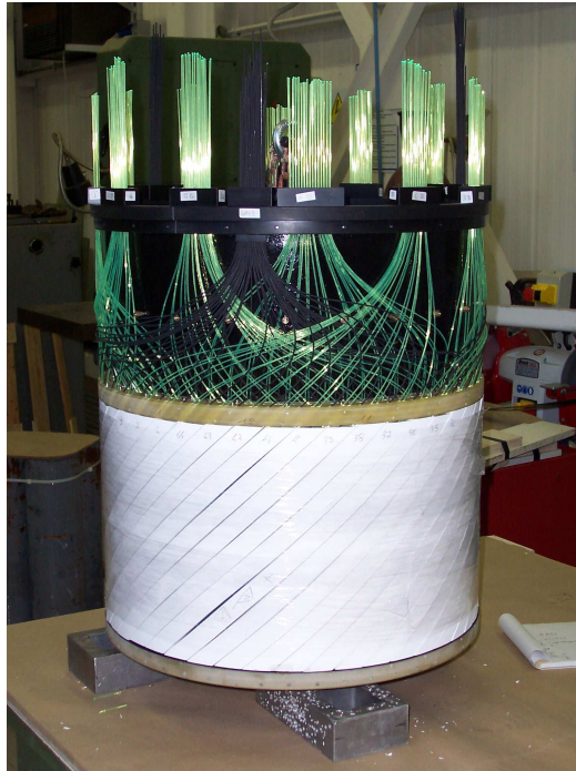
Figure 3.25: Assembling of the PD. The scintillator strips of the outer stereo layer are visible, as are wavelength shifting fibres and the connector rings.
