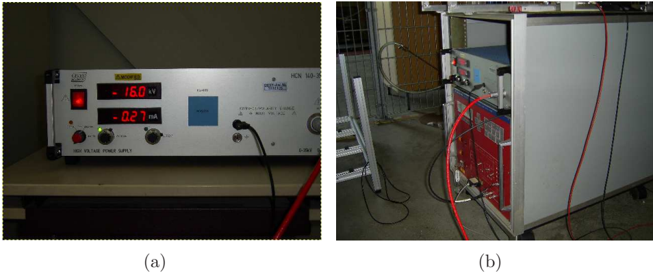
Figure 4.6: (a) shows a FUG HCN 140-35 power supply, which provides a maximum voltage of 35 kV and a maximal current of 4 mA. (b) shows a CAEN SY 527 multi channel power supply to power each GEM channel independently.
