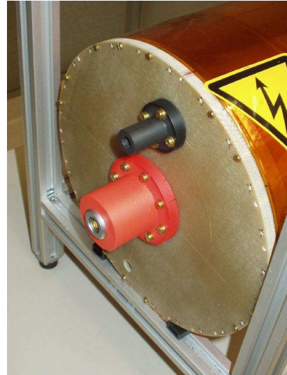
(b) Anode with the Prism Positioning System (c) Cathode with the quartz window
