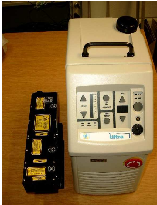
(a) The laser head and power supply of a UV CFR NdYag laser
