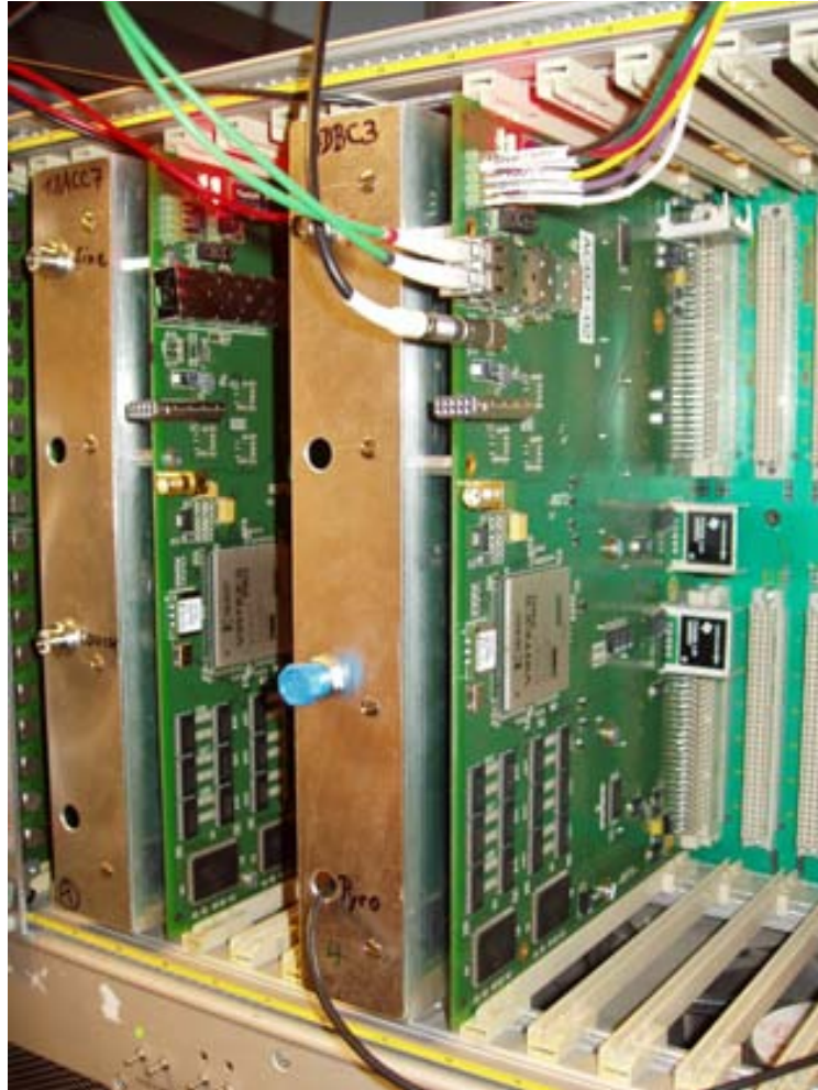
Figure E.5: BAM readout and regulation electronics. The aluminum chassis contains two photo detectors the signals of which are split and connected to two 16 bit, 108.3 MHz ADCs each. Adequate delays ensure that the two ADCs sample peak and baseline of the laser pulses coming from an optical BAM front-end. Alternatively, one of the four ADCs can be used to sample the signal of a bunch compression monitor. The FPGA installed on the VME board calculates the fast correction signals for the bunch arrival-time and bunch compression feedbacks. These corrections are sent via an optical RocketIO link (green cables) to the digital controller board of the first accelerating module ACC1.
