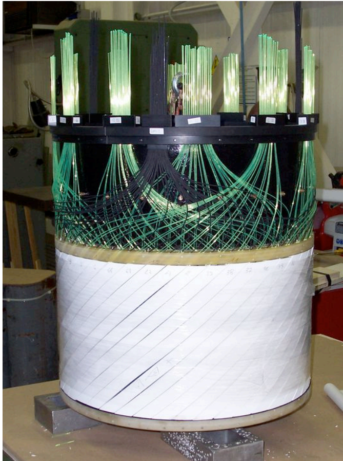
Figure 3.11: A picture of the fully mounted HERMES Recoil Photon Detector.
