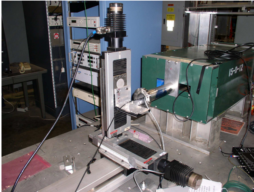
Figure 4.4: One of the 10D37 magnets on the test bench table during a B-field map. The beam pipe and one of the mirror plates mounted on one side of the magnet are also visible.
