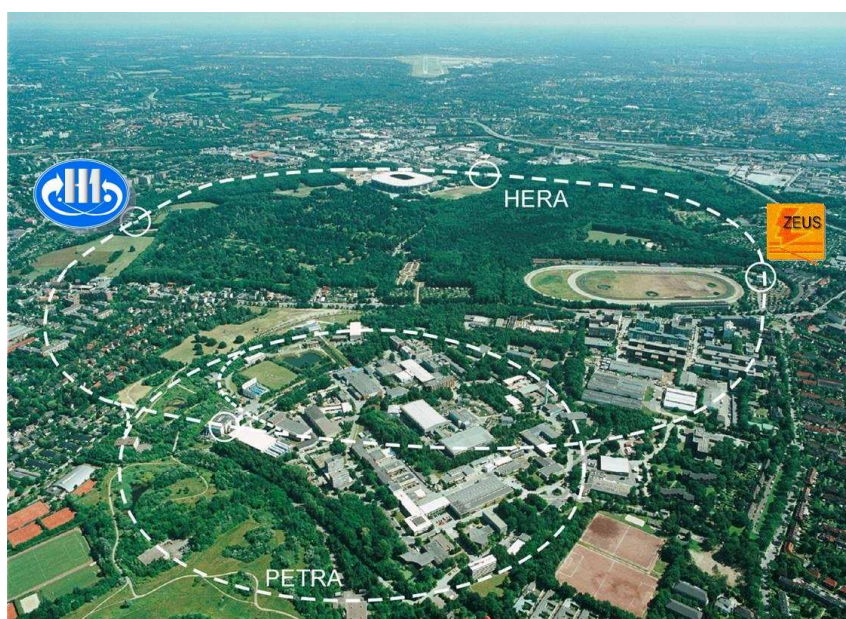
Figure 3.1: An aerial view of DESY. The main campus is the area encircled by HERA’s pre-accelerator PETRA (smaller dashed circle), the HERA collider (bigger dashed shape) extends beneath the Altonaer Volkspark and the Stadium. The HERA south hall with the ZEUS detector is off the main DESY ground, next to the Trabrennbahn.
