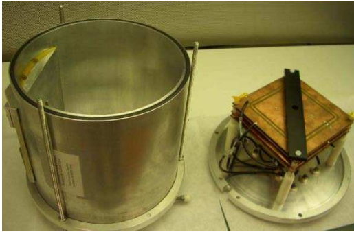
Figure 6.4: (a) Small TPC prototype, on the left the chamber is visible, on the right the inner assembly with the cathode and the source mounting on top of it is shown. (b) Medium size prototype [Die09].
