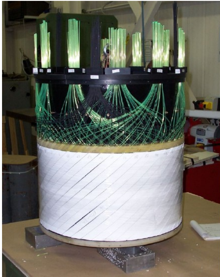
Figure 3.12: A picture of the photon detector [71]. The scintillating fibres are shown, as are the connection fibres to the readout electronics.
