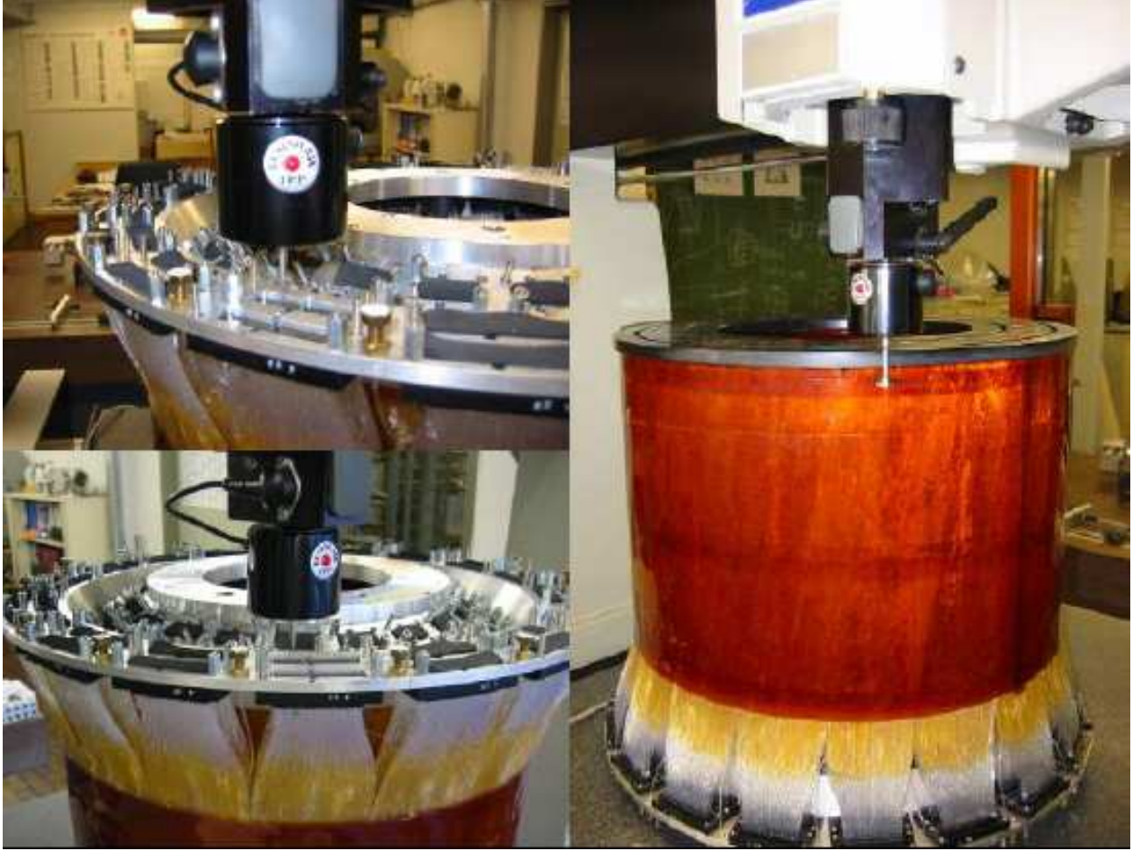
Figure 5.12: Photo of the measurement of the SFT at the Survey Group.
