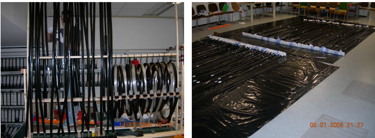
Figure 5.26: The left picture shows the support where the light guides were glued, the light guide should be glued with the fiber straight at the connector. The right picture shows the storage room in the East Hall. The light guides were stored as straight as possible to avoid damage, before the final installation.
