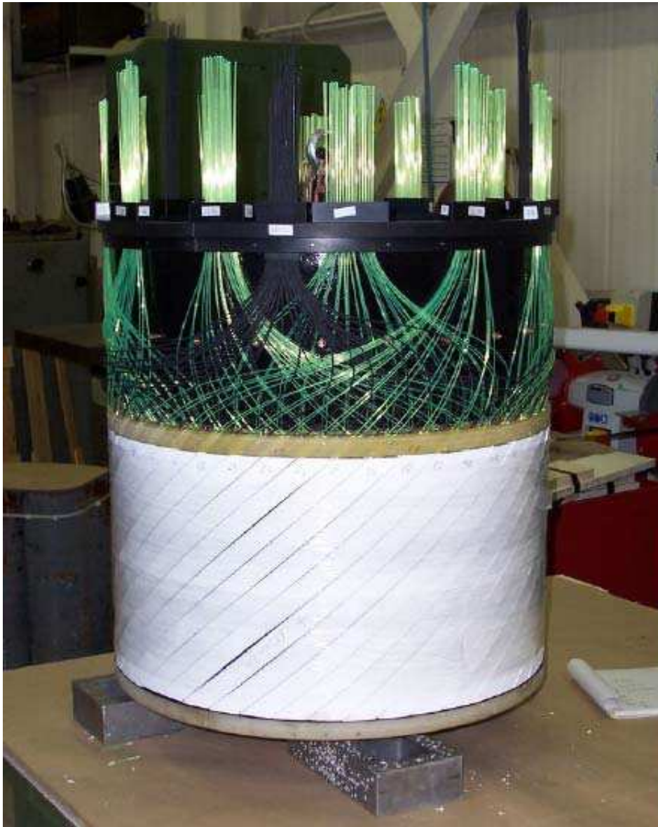
Figure 4.19: Photograph of the photon-detector. Internal setup of the Photon Detector during production and before mounting the light tide coverage. The green fibres of the wave-length shifters illustrate the three different orientations ( 0^\circ, \pm 45^\circ ) of the strip segments. The black fibres are used by the gain monitoring system [95].
