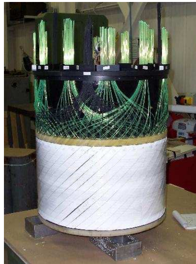
Figure 4.12: Picture of the photon detector during its assembly.
