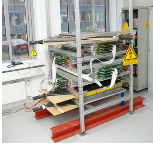
Figure 3.3: Setup of the muon tracker in the laboratory in Hamburg. The photograph shows the four drift tube modules placed on top of each other. Two of the modules are rotated by 90^\circ . The HV and preamp boards are placed at the front end of the modules (cf. Section 3.2.4 for details). The read out and control electronics as well as the power supplies are located in the rack behind the detector. On top and underneath the detectors, layers of plastic scintillators are placed for triggering. To reduce triggers from low energetic cosmic showers, a layer of lead is placed above the lowest scintillator.
