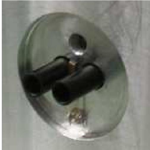
Figure 10.7: Detail of the LED mounting on the front u -leg. Visible are the two slender POM tubes, guiding the light from the LEDs in the two detector channels. The circular clearance allows the Cherenkov gas to flow freely between the two detector channels and the surrounding outer box volume. In between the POM tubes the temperature sensor is visible.
