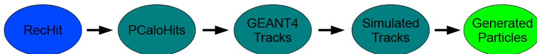
Figure 6.11: Flowchart for matching RecHits to generated particles - The matching is done by mapping the reference numbers (ID) of each of the objects. The simulated tracks are matched to the generated particles by comparing the particle ID in the track to the particle ID of the generated particle.
