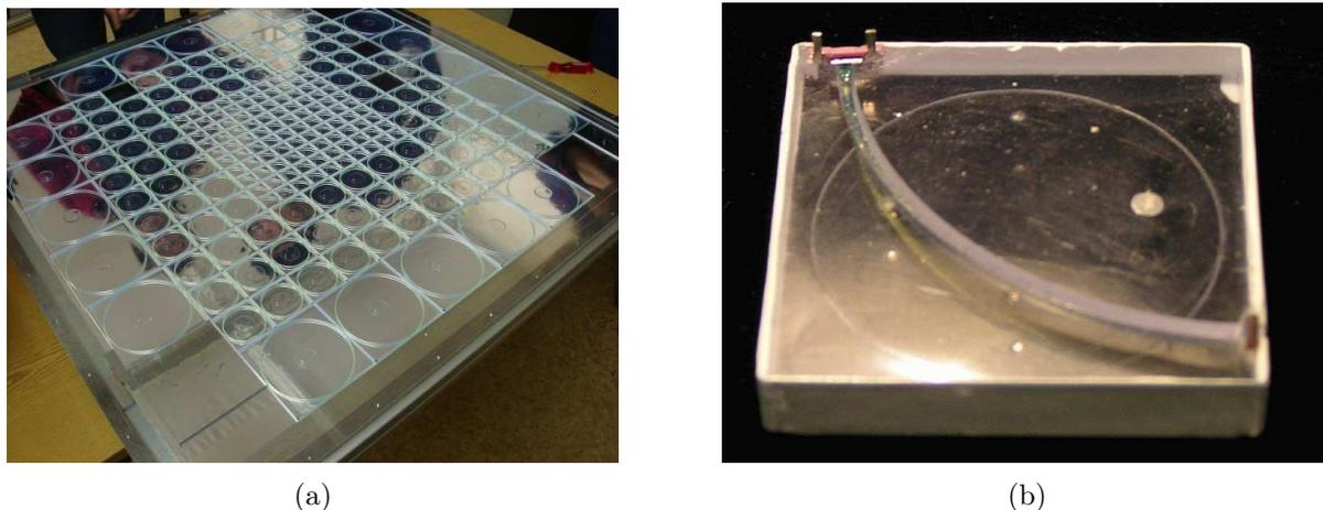
**Figure 2.6:** (a) A single AHCAL layer with 216 separate scintillator tiles [31]. (b) A  $3 \times 3 \text{ cm}^2$  scintillator tile with SiPM, mirror, and WLS [37].
