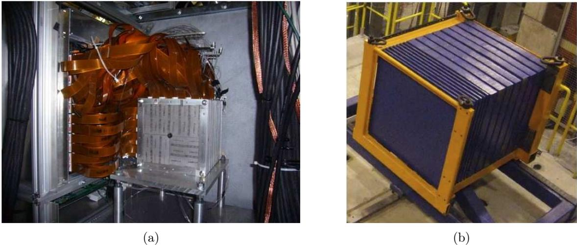
**Figure 2.5:** Pictures of (a) the Sci-ECAL [38] and (b) the TCMT absorber structure [39].
