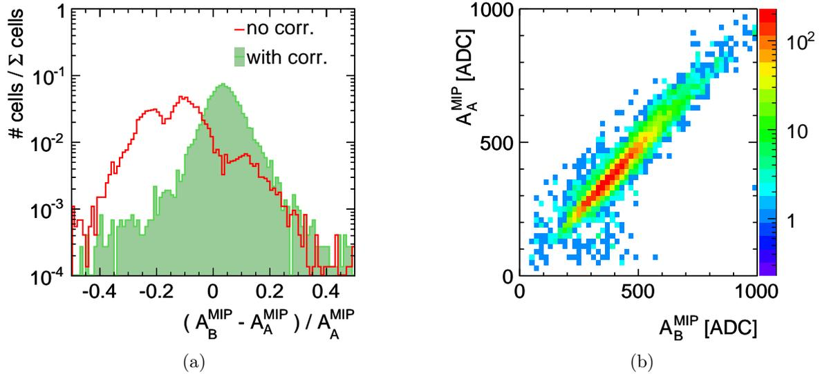
**Figure 4.4:** (a) Difference between native ( $A_A^{\text{MIP}}$ ) and non-native ( $A_B^{\text{MIP}}$ ) muon calibration factors before (open histogram) and after (filled histogram) correcting for the effects of voltage and temperature differences. (b) Correlation between the native and non-native muon calibration factors after correcting for the effects of voltage and temperature differences.
