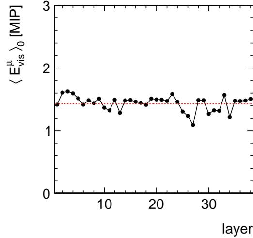
**Figure 4.3:** Mean AHCAL response  $\langle E_{\text{vis}}^\mu \rangle_0$  per layer for muon measurements after subtracting the mean noise per layer (extracted from random trigger events). The dashed line marks the mean response of all layers (1.43 MIP).
