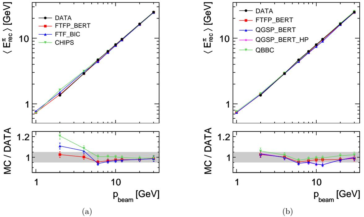
**Figure 8.5:** (a-b) Mean reconstructed energy  $\langle E_{\text{rec}}^{\pi} \rangle$  for pion data and Monte Carlo simulations using different GEANT4 physics lists as a function of the pion momentum. The ratios between the predictions from simulations and data are presented as well with gray bands indicating the range of 5% agreement.
