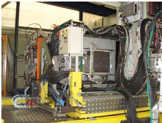
**Figure 3.4:** Picture of the integrated detector setup with the Si-WECAL (front), the AHCAL (center), and the TCMT (back). The Si-WECAL and the AHCAL reside on the movable stage. Part of the DAQ commonly used by all three calorimeters is visible on the right.
