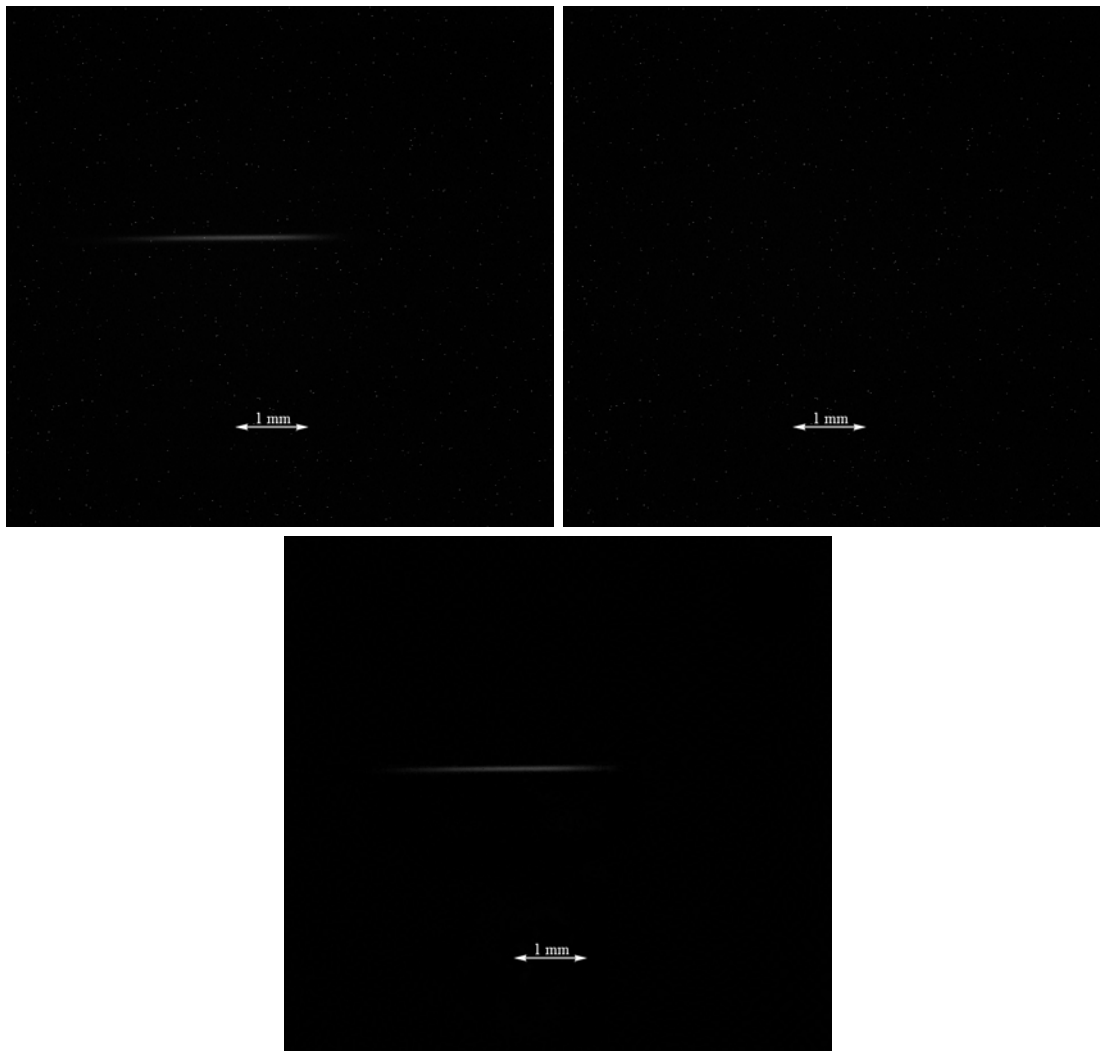
Figure 7.6.: Convolution of Laser intensity distribution and the efficiency of the imaging system: On the left the raw data (with gas supply), on the right the background signal and below the background subtracted intensity. The pictures were taken without the capillary to measure just the laser intensity distribution.
