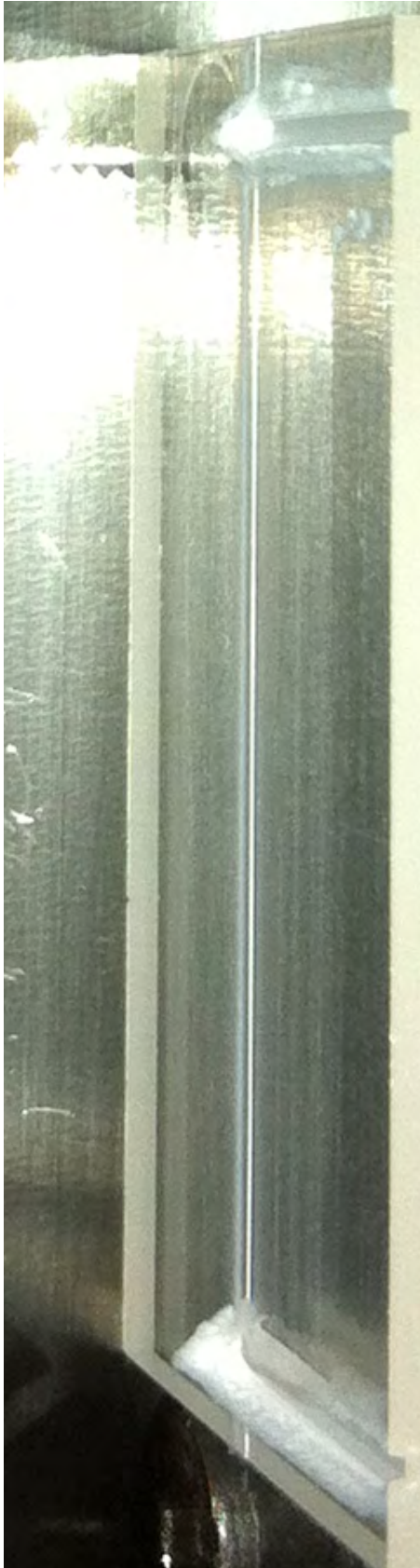
Figure 5.1.: Machined capillary half with gas inlets. At the inlets the deposition of the ejected dusty material can be seen which is easily blown away by any kind of airflow.
