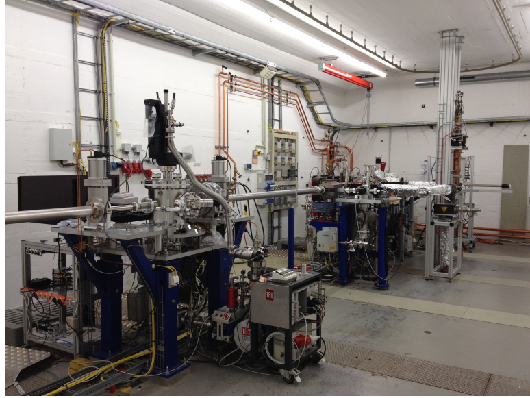
Figure 1.3: Photo of the REGAE linear electron accelerator. On the left: the target chamber, on the right: the accelerator section.
