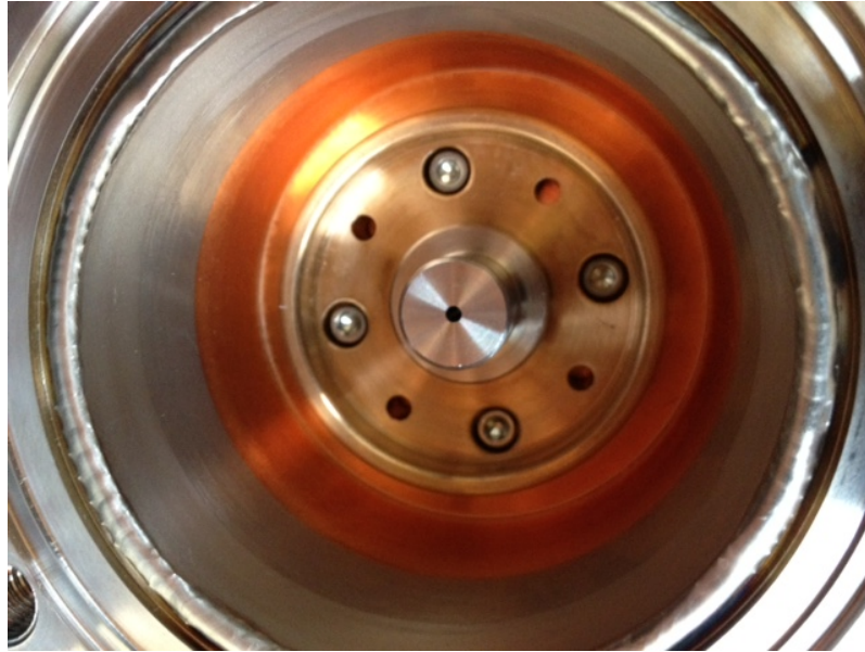
Figure 2.31: The new cathode holder with an inserted cathode dummy.
