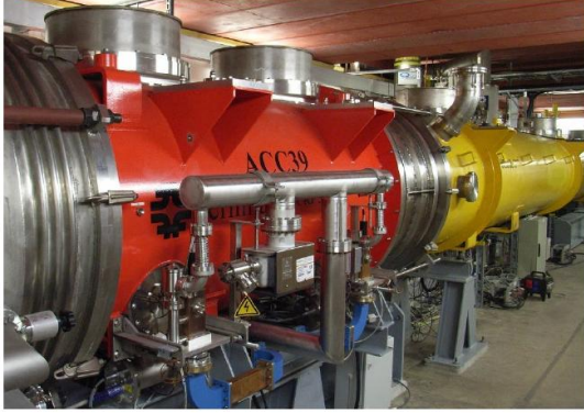
Figure 1.7: ACC39 module (red) in FLASH. The module in yellow, on the right, is ACC1. The direction of travel of the multi-bunch beam, is from right to left.
