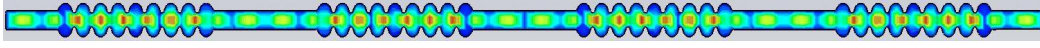
Figure 2.15: The electric field distribution of the strongest coupled cavity mode from the first dipole band (frequency: 4.8076 GHz, R/Q : 125.762 \Omega/\text{cm}^2 per module). Electric (EE) boundary conditions were used in the simulation.
