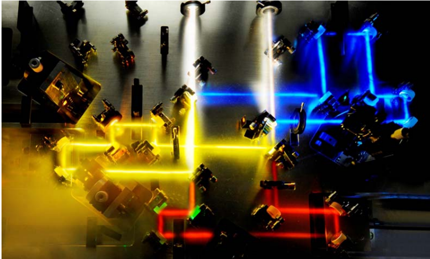
Fig. S3 Photograph of the field synthesizer in operation. Beams have been visualized by nitrogen vapor.
