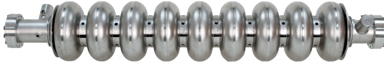
Figure 3.5: Nine-cell niobium cavity. About 7400 of these cavities per beam accelerate the electrons and positrons to an energy of up to 250 GeV. Figure taken from [55].
