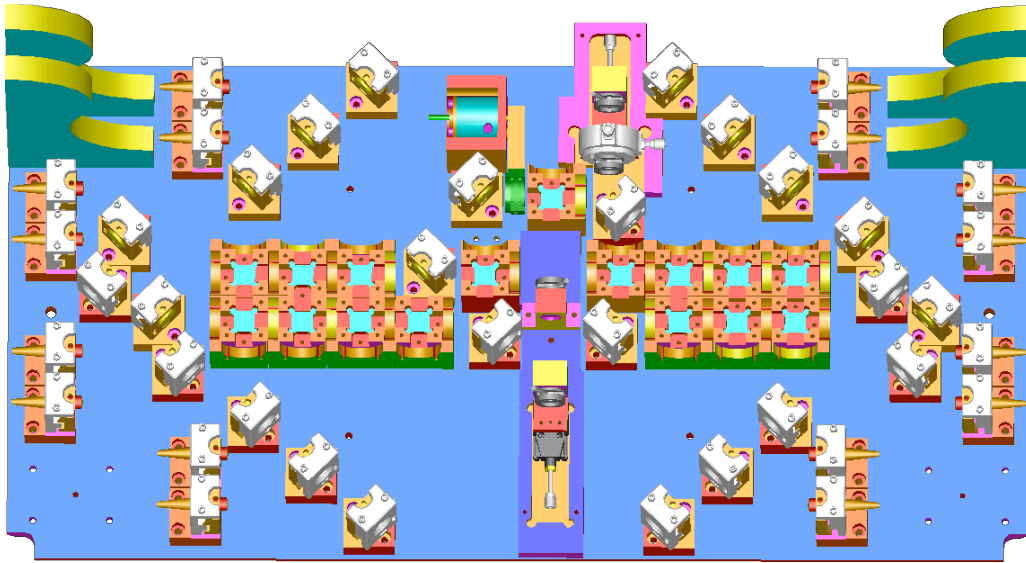
Figure G.3 | 3D CAD model of the free-space distribution unit. The device is shown in its slightly upgraded version “1.1” with more stable mirror mounts compared to the original design.
