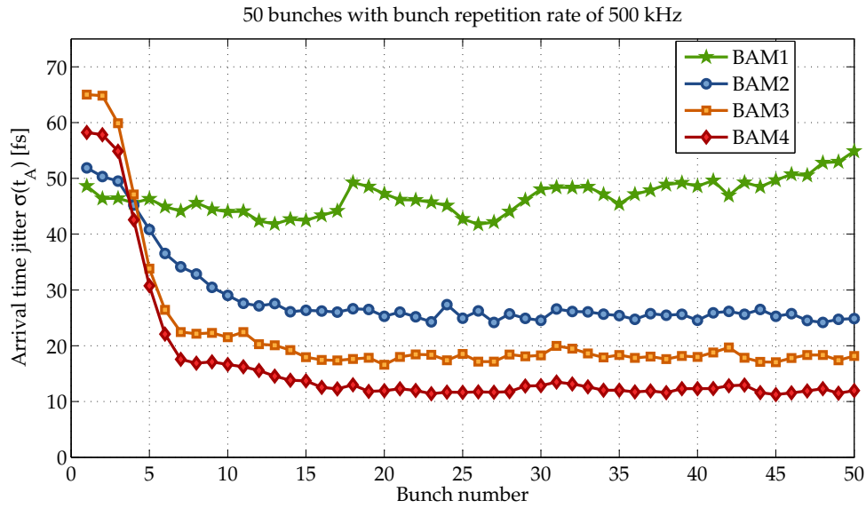
Figure 5.1.13: Standard deviation of bunch arrival time with applied beam-based feedback to ACC1 and ACC23 at FLASH.
