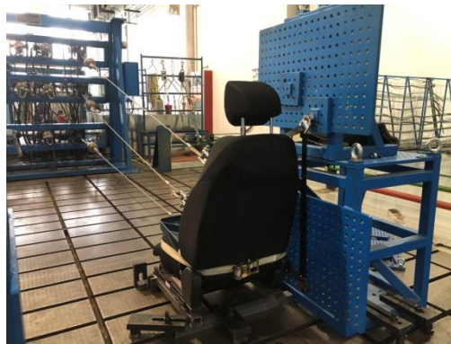
Figure 5. The picture of seat anchorage strength test.
