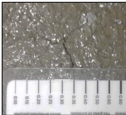
Figure 6. 0.35 mm fissure.
