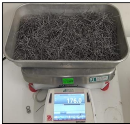
Figure 1. Recycled polypropylene fibers
