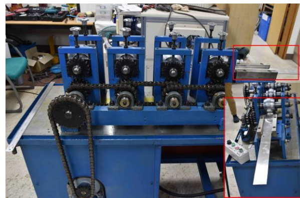
(b) Roll forming test setup
