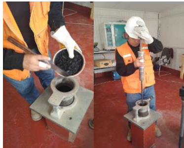
Figure 6. MAC is placed left fresh from the oven in the Marshall test specimens, which are struck an average of 75 times around the mold.
