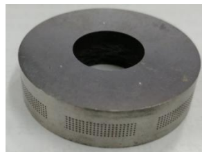
Figure 2. Lower test piece with circular microstructures
