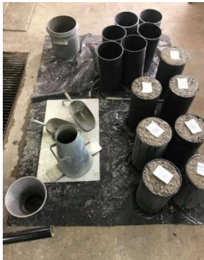
Figure 1. Specimens concrete 6''x12''
