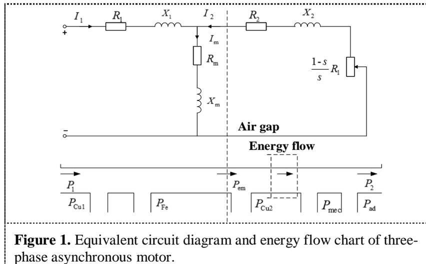
**Figure 1.** Equivalent circuit diagram and energy flow chart of three-phase asynchronous motor.
