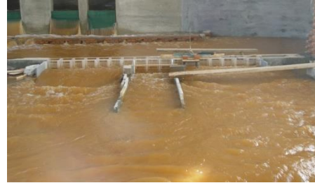
Figure 5. Comparison of the hydraulic jump characteristics between the roughened-bed stilling basin and the traditional smooth-bed stilling basin.
