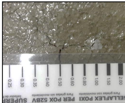
Figure 4. 0.50mm fissure.
