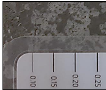
Figure 9. 0.10 mm fissure.
