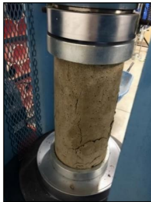
Figure 4. Compressive Strength Test
