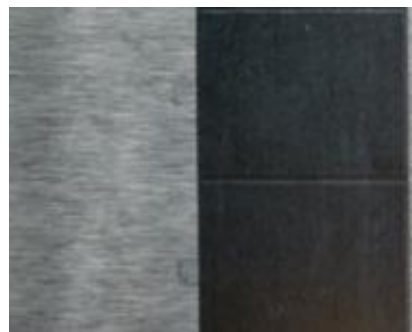
Figure.4 Die steel before and after laser polishing
