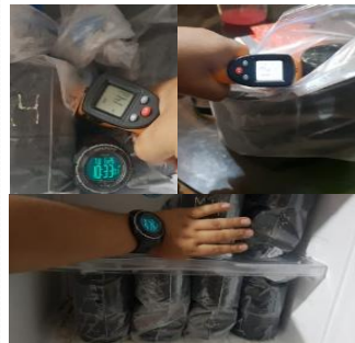
Figure 7. The specimens are frozen for 24 hours. Simulating extreme climates where they can be placed [4]
