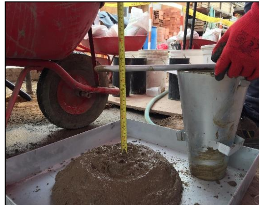
Figure 5. Slump Test
