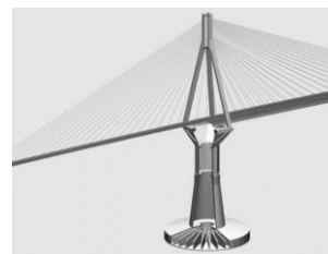
Figure 14. Super-large diameter hollow single-tubular column foundation of Rion-Antirion [22]
