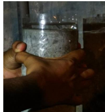
Figure 2. Specimen in water permeability test
