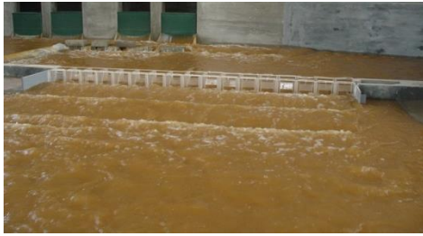
Figure 4. The secondary hydraulic jump generated after the end of the traditional smooth-bed stilling basin.
