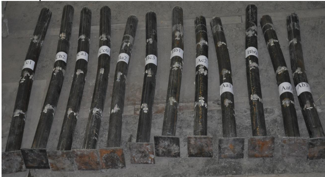
Fig.1. Potograph of specimens failure mode
