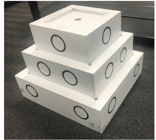
Figure 6. The prototype of the tower calibration pattern.
