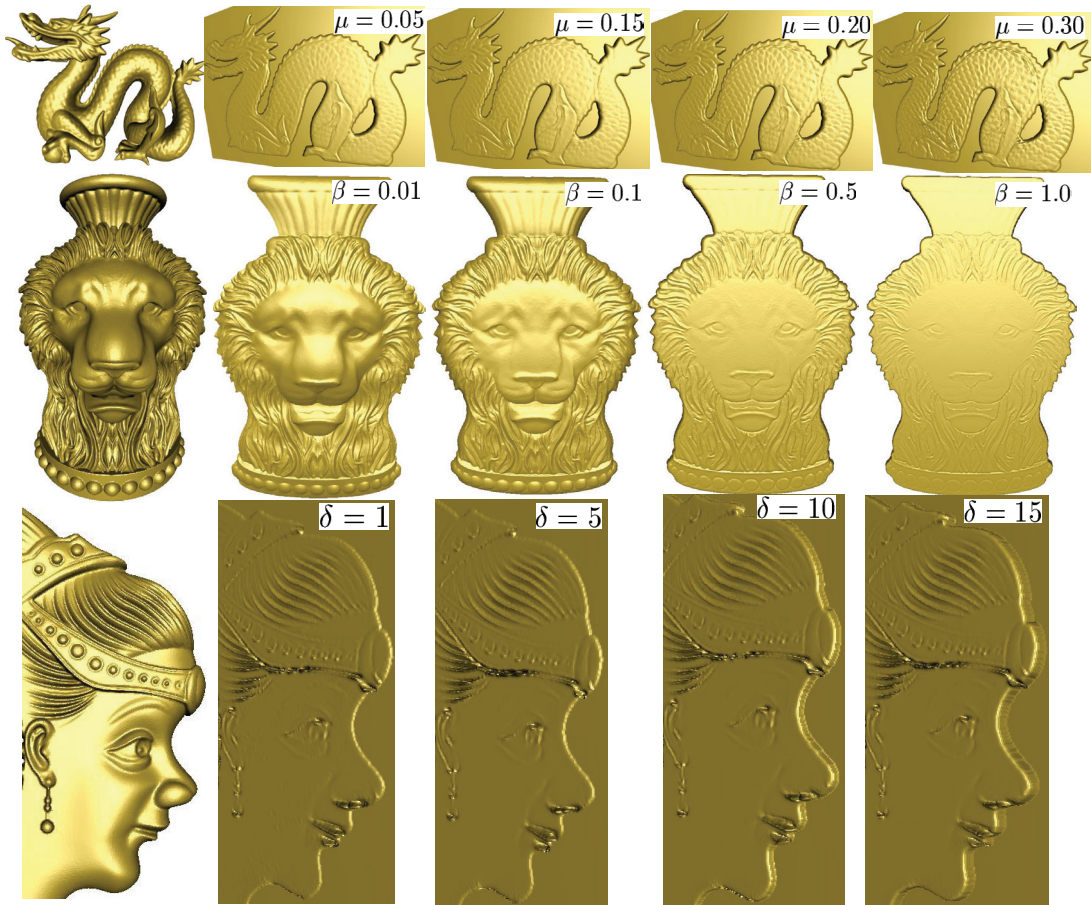
Figure 7. The bas-relief modeling method has three vital parameters. The first row shows that details can be increasingly enhanced by enlarging \mu when the other two parameters are fixed, i.e. \beta = 0.3 , and \delta = 10 . The second row means that enlarging \beta can obtain flatter bas-reliefs ( \mu = 0.15 , \delta = 12 ). The third row illustrates that enlarging \delta produces bas-reliefs with higher heights ( \mu = 0.01 , \beta = 1 ).
