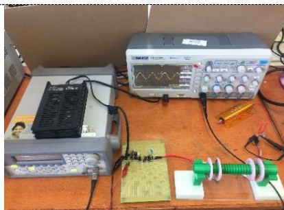
Figure 7. Experiment platform of the wireless power transfer.
