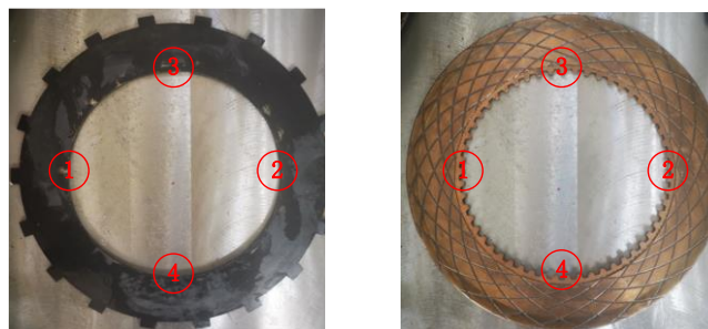
Figure 3. Measured points of the clutch disks
