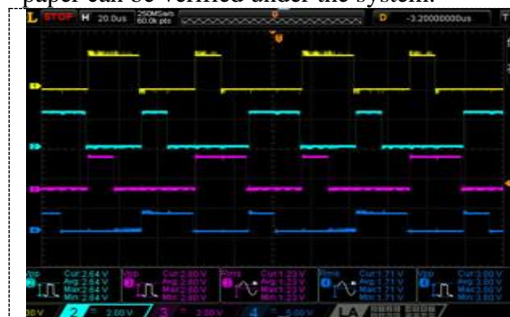
Figure 5. PWM drive waveform output from hardware
