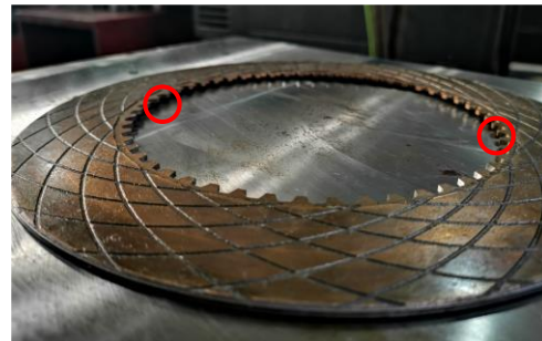
Figure1. 3D sketch of the clutch system Figure 2. A typical deformation of the friction disk
