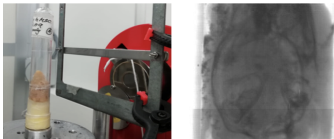
Figure 7. Left: nude mouse head in PMMA container, right: one offset and gain corrected projection of the mouse head.
