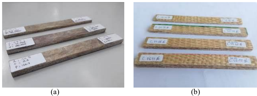
Figure 5. Samples of abaca composite specimen (a) with stitched random orientation fiber, (b) plain weave woven fiber.
