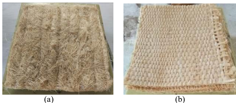
Figure 2. The abaca fiber (a) stitched random orientation, (b) plain weave woven.
