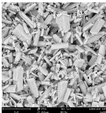
Figure 3. SEM micrographs of Gallium Oxide bulk powder.
