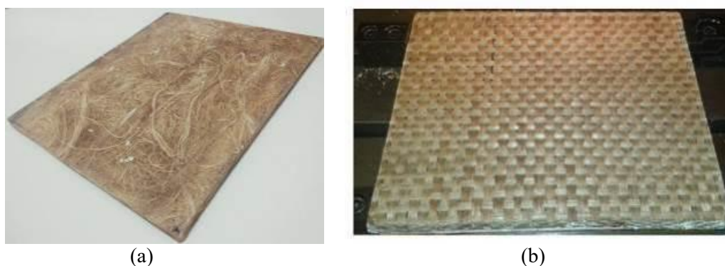
Figure 4. Abaca composite panels (a) with stitched random orientation fiber, (b) plain weave woven fiber.
