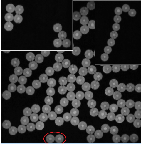
Figure 4. The main picture shows the last frame from an experiment with 144 particles. A dimer separate from the main cluster is highlighted by a red ellipse. The insets show the last frame for two separate experiments with nine particles.
