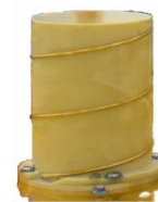
Figure 5. The ADS-B antenna on TT-3.
