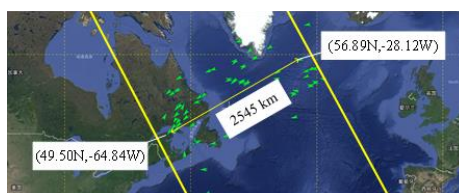
Figure 6. Sketch map for detection width analysis of TT3-ADS-B.
