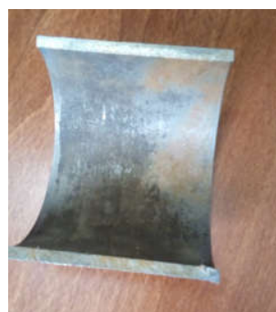
Figure 2. Cut worn shaft sleeve inner surface.
