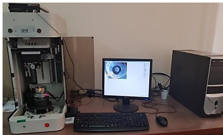
Figure 6. General view of the CETR UMT 2 Tribometer.
