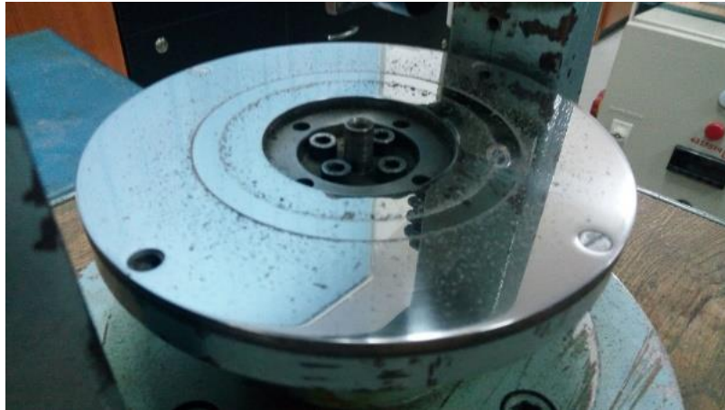
Figure 4. Residue left on disc after a wear test.
