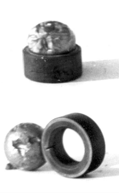
Figure 2. Some examples concerning the working damage of valves.
