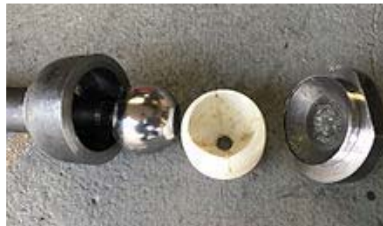
Figure 2. Spherical joints from motor vehicle industry [8]
