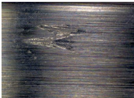
CoCrWMo ring surface after lubricated test (30 N)
