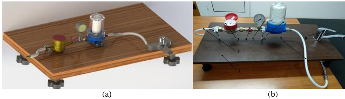
Figure 1. (a) CAD model of the experimental stand, (b) Experimental stand developed.
