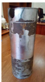
Figure 1. Worn shaft sleeve outer surface.
