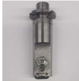
Figure 3. The chain link mounted in the holder.
