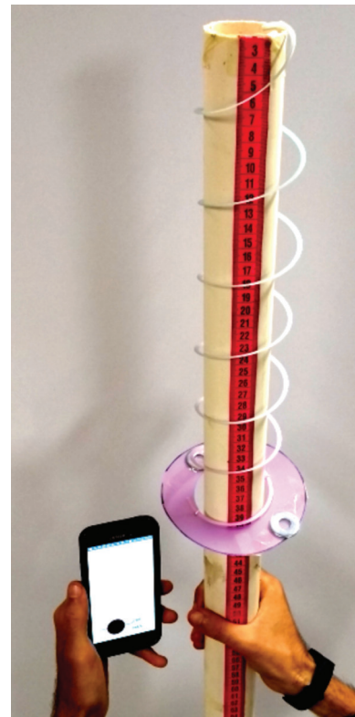
Figure 4. Experiment to be performed in groups of students. The spiral toy is fixed to the top of the guiding white tube. The oscillations are read against the cloth tape in red. The pink plastic ring and the metal washers attached to it change the oscillator damping factor and mass, respectively.
