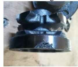
Figure 5. Product hole defects on the surface
