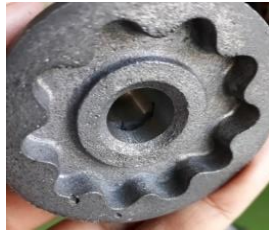
Figure 2. Pinhole crack defective product
