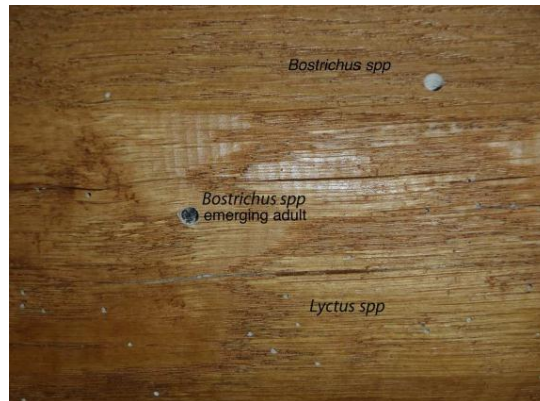
Figure 2. Surface holes due to Lyctus spp. attack and B. capucinus attack [15].
