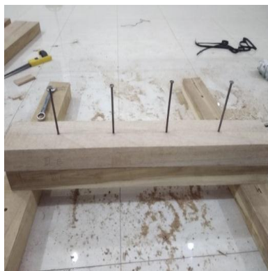
Figure 2. Nail instalation
