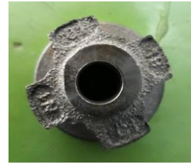
Figure 3. Defective products of imperfect casting
