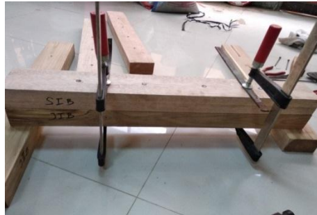
Figure 1. Laminated beam between teak wood at the bottom and sengon wood at the top
