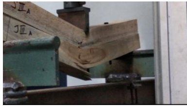
Figure 8. Failure Pattern of Lamination Beam using bolt connector.
