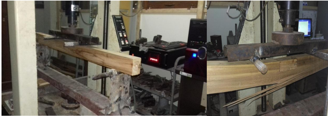
Figure 9. Setting-up Flexural Strength of Retrfitting Wood Beam.
