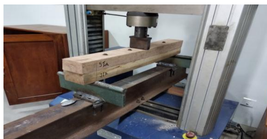
Figure 4. Settingup of flexural testing
