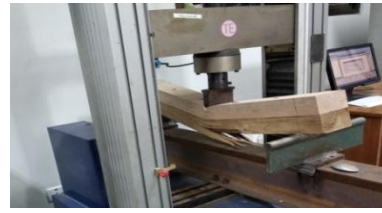
Figure 9. Failure Pattern of Lamination Beam using nail connector
