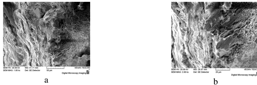
Figure 9. Room temperature tensile fracture scanning electron microscope - a-1000X, b-2000X
