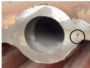
Figure 1. Incomplete penetration fin weld
