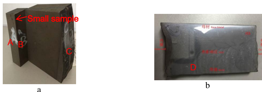
Figure 1. Metallographic sample; a crack tip; b pipe cross section
