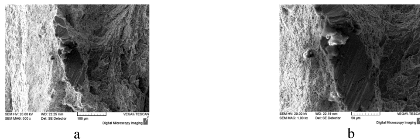
Figure 8. Scanning electron microscopic observation of the cracking zone of impact specimen ZCJ3—a-500X, b-1000X
